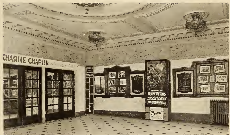
Not a new idea, but a good one when one-sheets are worth featuring as an advance display. The frame for the Universal paper on "The Storm," used in the lobby of the Merrick Theatre, is a shadow box, illuminated by an electric lamp connected by a flexible wire with the lobby fixture. A simple arrangement and a device which can be used over and over again.
