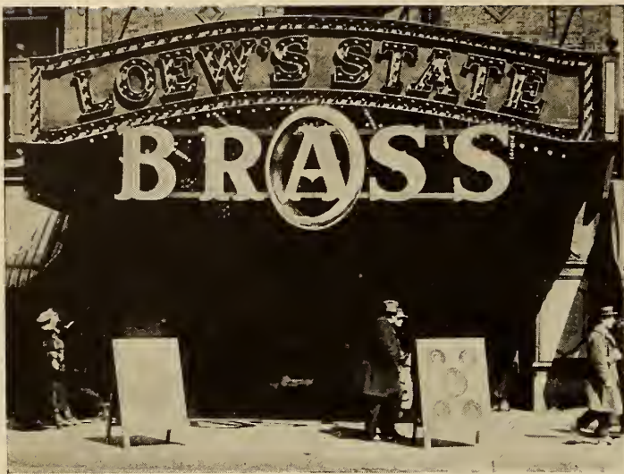
The cut-out letters of "Brass," on the marquee of Loew's State, Buffalo, for the engagement of the Warner Brothers' feature, were of compo board covered with metallic paint. The wedding ring around the letter "A" is an old automobile tire, also covered with the brass paint.
