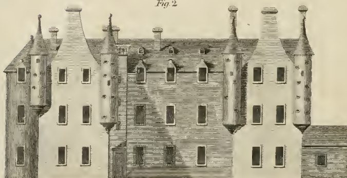
Elevation of a variety of the Turret style common in the neighbourhood of Edinburgh.
