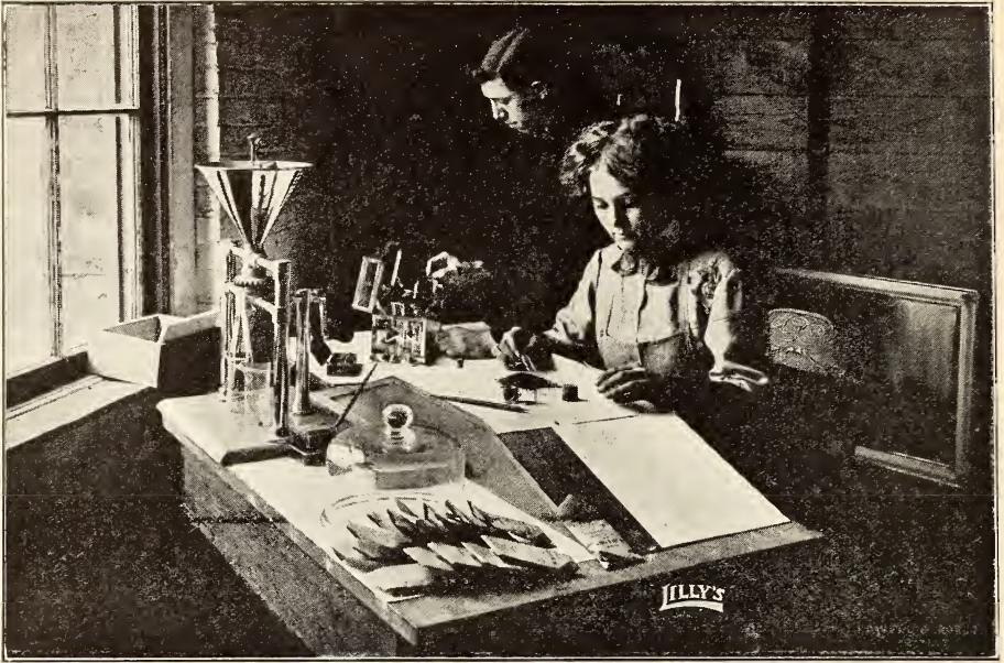
This picture shows the instruments used by The Chas. H. Lilly Co. for making seed analysis for purity. The Mixing Machine thoroughly mixes samples from different parts of each bag of each lot of seed, thus insuring a fair sample. The Scale is a very delicate instrument, will show the weight of the tiniest seed, and must be enclosed in a glass case. The operator must be an expert, and be able to name every seed in the sample.
