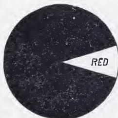
FIG. 91.—Disk with 10 Parts Vermilion and 90 Parts Black: gives by rotation a dark-reddish chocolate-brown.
