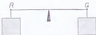
FIG. 97.—Along the line R G we can arrange all the mixtures of red and green. The diagram represents the case where equal parts of red and green are employed. Then the point of support (mixture-point) must be in the centre of the line R G.
