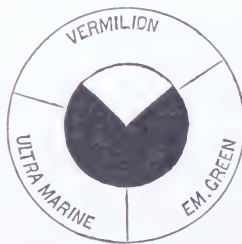
FIG. 101.—Compound Disk of Vermilion, Emerald-green, Ultramarine, White and Black, arranged for the production of Grey.
