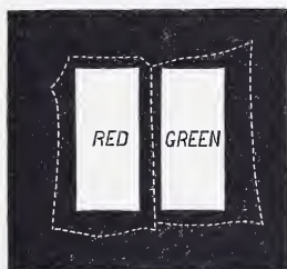
FIG. 58.—Two Apertures in Black Cardboard covered with Red and Green Glass (natural size.)
