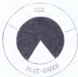
FIG. 53.—Large Disk of Red and Blue-green arranged for the Production of a Pure Grey, Small Disk of Black and White furnishes the same Grey
