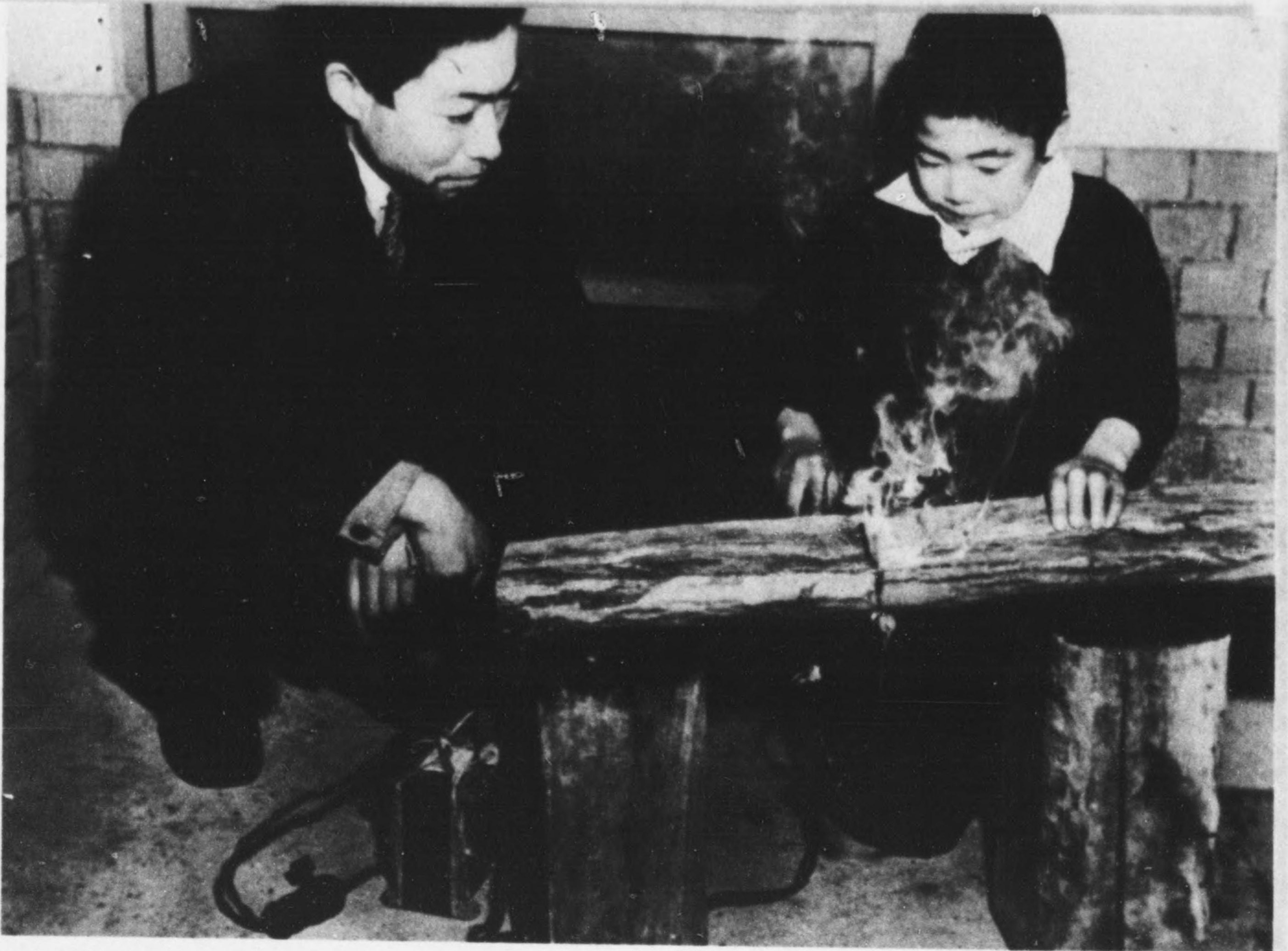
ADVANCEMENTS IN INDUSTRY . . . Dr. Yoshimitsu Kikuchi watches the operation of a new type of electrical wood-cutter saw which he has invented. The saw operates on the principle of an electrically heated wire which cuts through the wood by its burning action.
