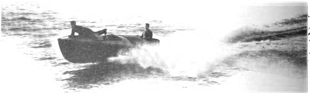
"BUG," THE KING OF SIXTEEN FOOTERS THIS 16-FOOT HYDROPLANE IS CAPABLE OF 30 MILES PER HOUR WITH A 40-HORSEPOWER ENGINE
