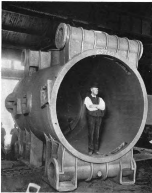
ONE OF THE TWO LOW PRESSURE CYLINDERS OF THE "SEE-AND-BEE." THEY ARE EACH ABOUT 13 FEET LONG AND WEIGH OVER 32½ TONS—ONE OF THE LARGEST SINGLE CASTINGS EVER MADE.
