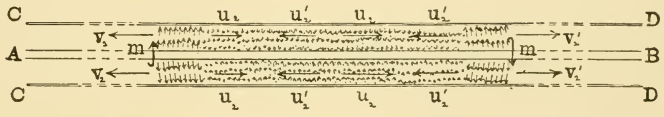
FIGS. 20-22.—Movement of Electric Flux in Cable of Imperfect Insulation and Perfect Conduction.
