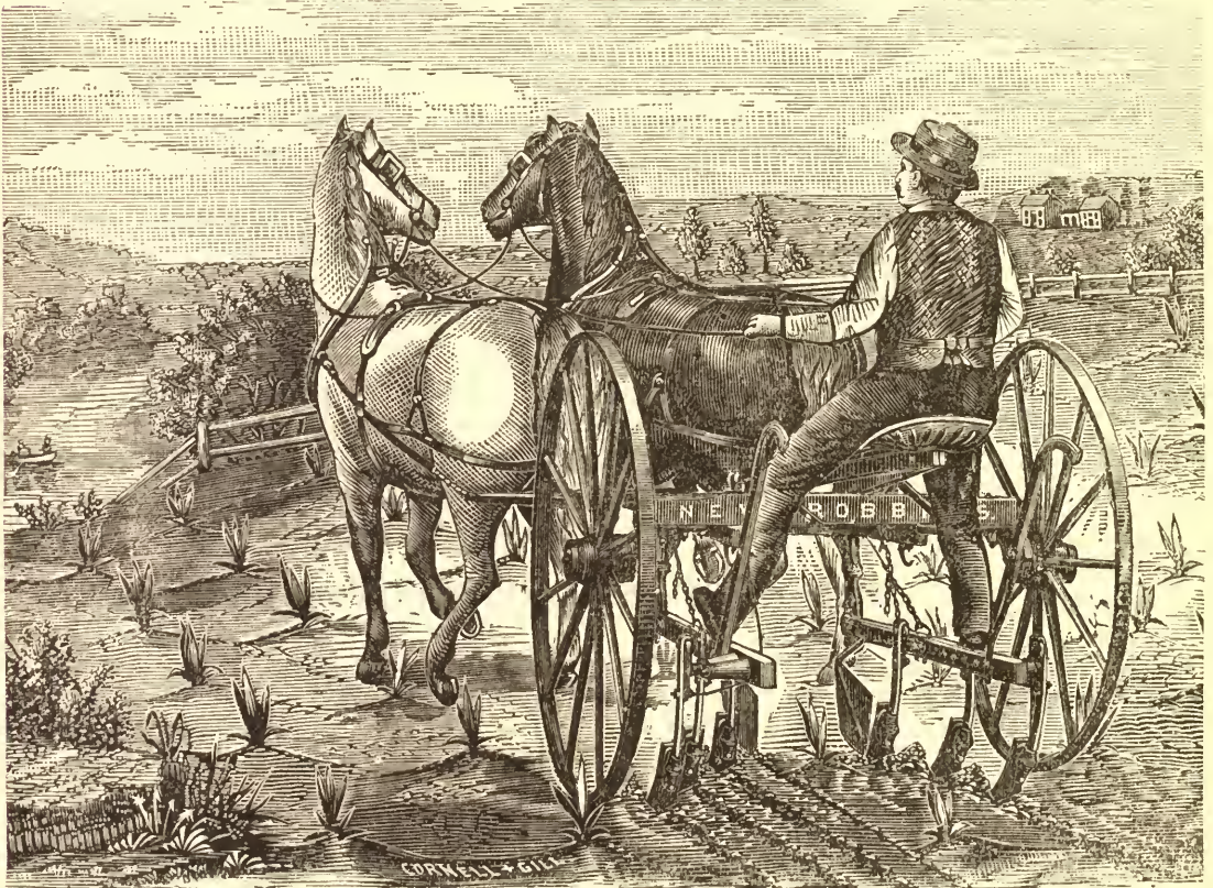
THE ROBBINS CULTIVATOR, ADJUSTED FOR CORN.
