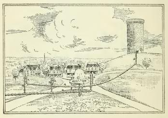
FIGURE 60.—Water-tank, water-pipes, and sewer-pipes for a town. The water-pipes are shown as lying at a higher level than the sewer-pipes. Of course, both are underground in all towns and cities.
