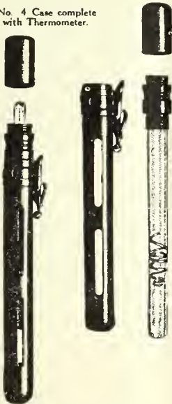
At the left, the outside case. Above, the glass tube with spring and the screw lock cap.
