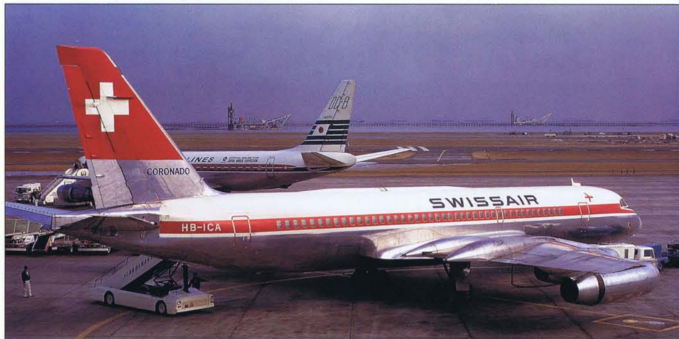
"A" model upgrades visible on HB-ICA include engine pod extensions and an enlarged wing fillet. (N. Williams via Terry Waddington)
