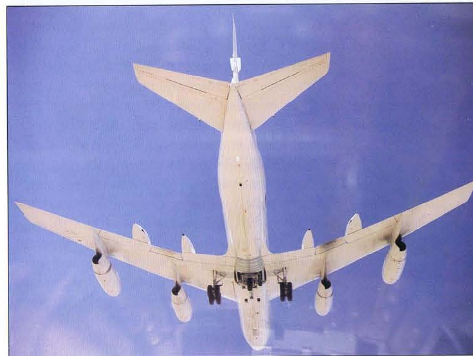
Highly modified LSRA in flight, showing the space shuttle test landing gear installation. Note that the Convair's main wheels are permanently locked down while the nose gear is retractable. Also visible are the nacelle inboard terminal fairing spats adopted during A model conversions on American Airlines 30A-5 examples. Blade radio antenna protrudes from the vertical stabilizer. (NASA)
