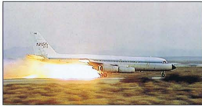
Among the last tests was this "roll-on-rims" drill (left) conducted on an Edwards concrete runway that produced dramatic results. Tire failure parameters tests (below) using the dry lake bed were less spectacular. (NASA photos)
