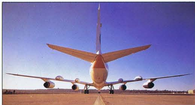
Above: Convair's new design featured fatter engine pods and unique wing-mounted anti-shock bodies. Below: The outer anti-shock body fuel dump chute can be seen along with the unmodified engine nacelle. (General Dynamics photos)
