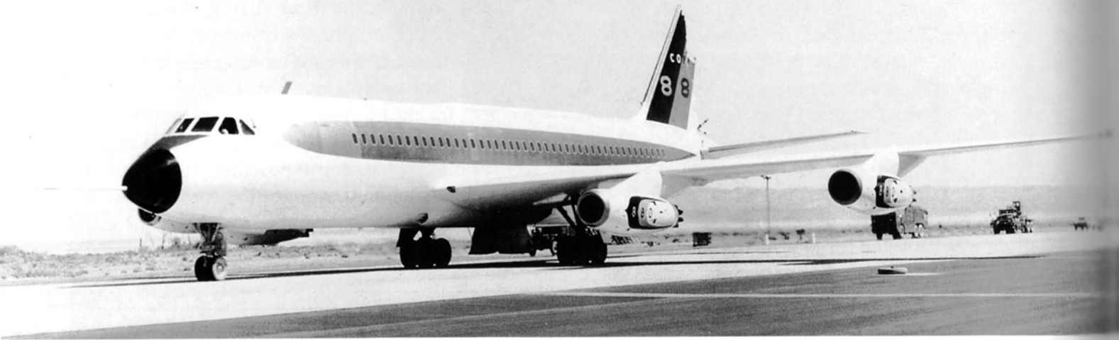
Ship One made an unplanned appearance at Edwards Air Force Base with its rudder missing and vertical stabilizer nearly torn away following flutter tests over the Pacific. Note the unusual engine nacelle logo symbols. (Edwards Air Force Base Archives)
