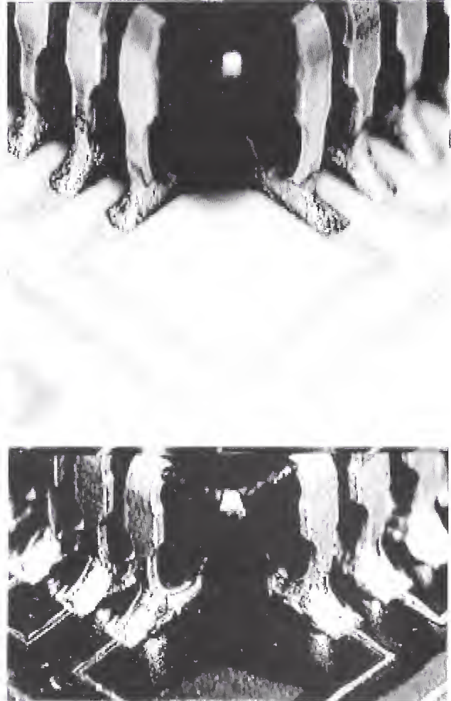
Figure 1. Plastic leaded chip carriers on ceramic (top) and polymeric (bottom) substrates assembled with Pb-free solders and surface finishes.
