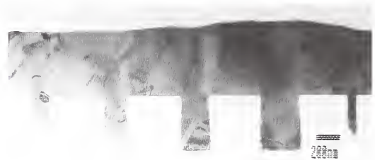
Figure 2. TEM image of copper electrodeposited nanoscale features in "superfilled" trenches. The electrodeposited copper contained microstructural defects such as voids, dislocations and twins that could not be revealed in the focused ion beam imaging.
