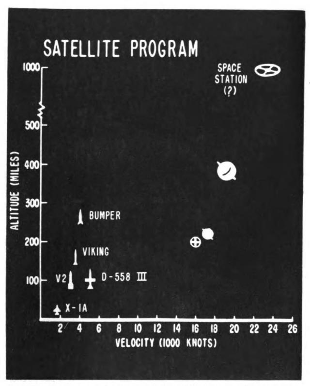
Above chart shows progress being made with rockets and illustrates tremendous speed which must be attained to establish a space station which would orbit the earth. A three-stage Redstone rocket was fired over Atlantic in late 1956. It traveled 3000 miles, went 400 miles up.
