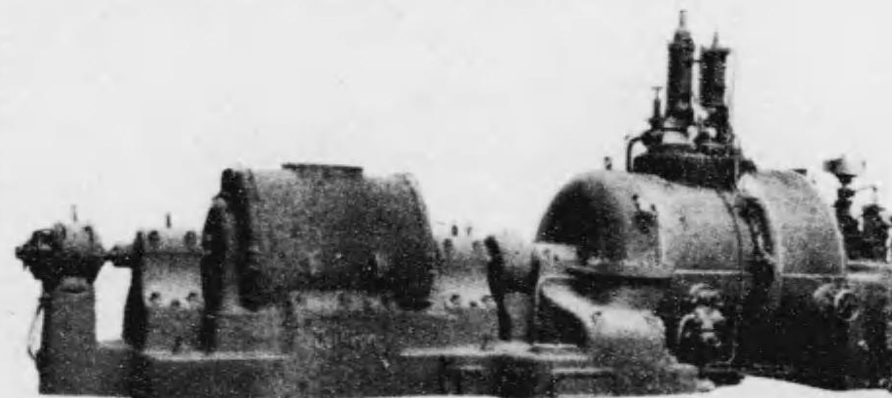
1000 B. H. P. by-pass Turbo-Generator, constructed for the extraction of heating steam at two different pressures, supplied to Societe Electro-Metallurgique Gardanne.
