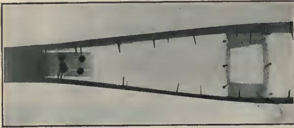
FIG. 4.—Radiograph of aeroplane hollow "box" strut, showing badly fitting internal end-block split by screws. (Kaye and Knox.)
