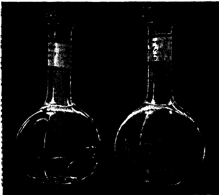
FIG. 3.—Flasks after incubation, showing colloids on film of gelatine with which the inner surface is coated.
