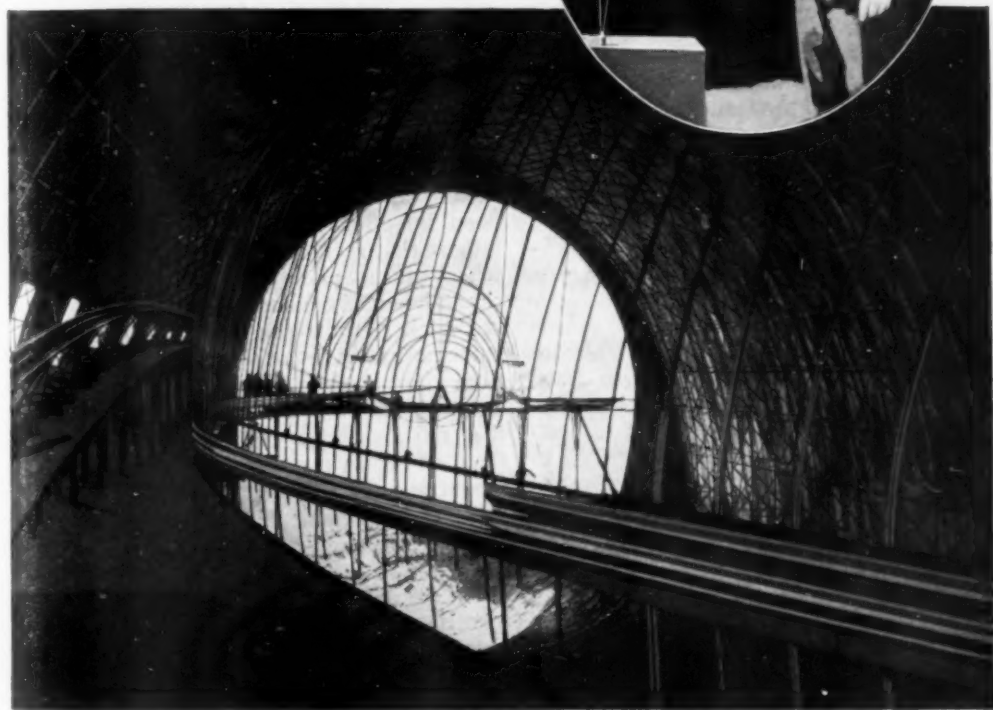
Framework of a Metal Dirigible under Construction in the Hangar, and a Model of the Ship, with Its Designer; the Builders Work from the Movable Platform in the Foreground
