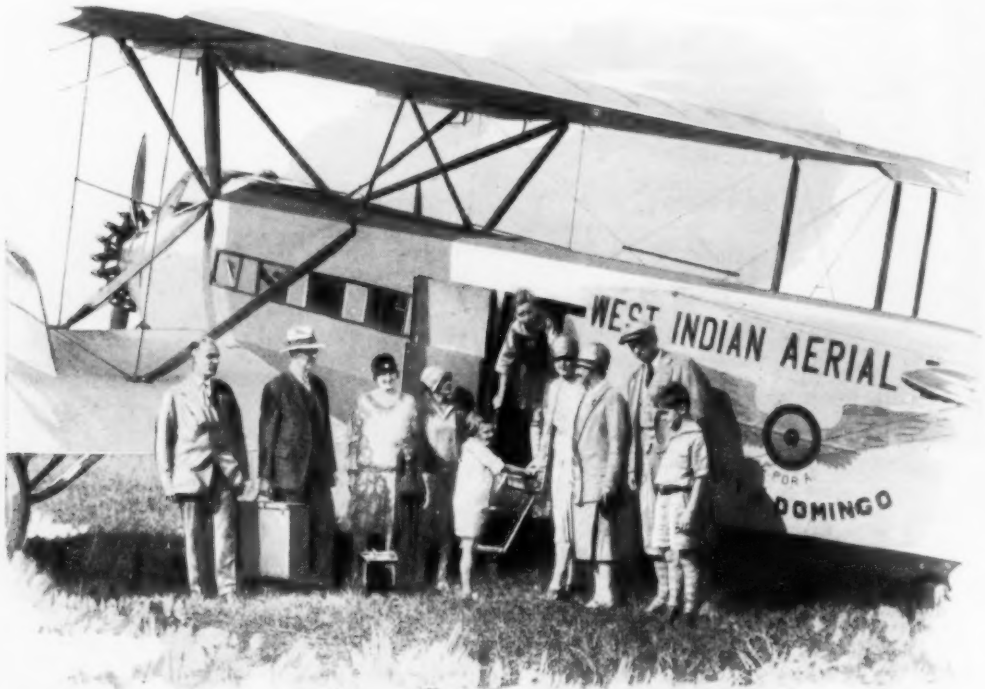
This Big Three-Motored Keystone Plane, Carrying Ten Passengers, Has an Insulated Cabin to Keep Out the Heat of the Tropical Sun, For It Flies the Caribbean Route
