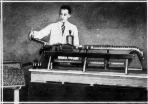
Machine Which Seals Bottles with Ordinary Glue Instead of the Usual Wax
