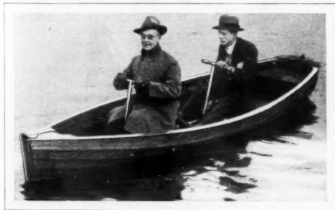
Boat Driven by Propeller Which Is Turned by Pumping Hand Levers, Much Like a Railroad Handcar
