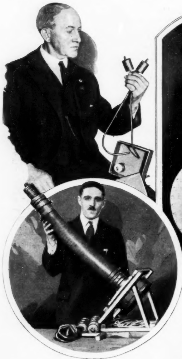
Upper Left, Float Apparatus to Establish Telephone Communication from Sunken Submarines; Right, Section of Steel Tubing to Reach Craft, and, Below, Model of Food and Water-Supply Tube
