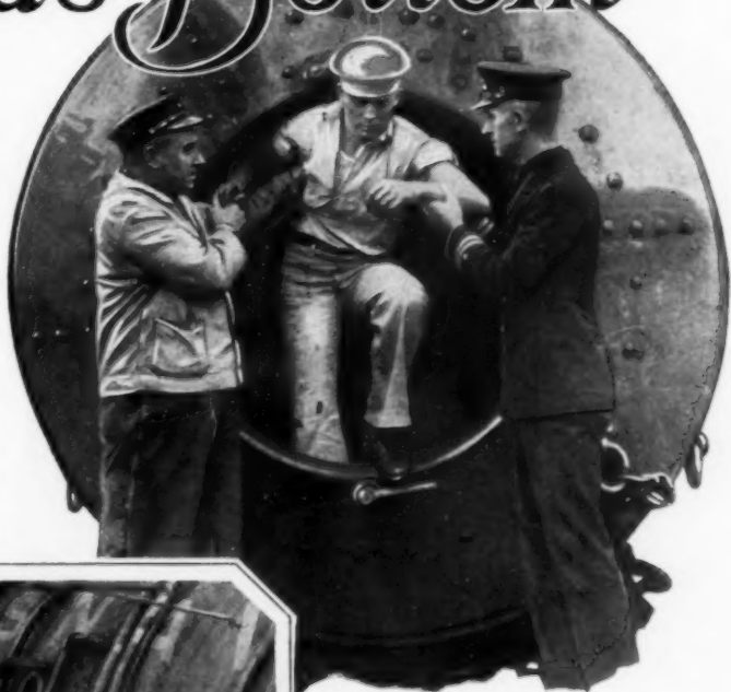
Assisting a Diver from the Pressure Tank after Treatment to Prevent the "Bends," and, at Left, Sailors on Duty at the Tank Controls, Slowly Lowering the Air Pressure in Its Interior
