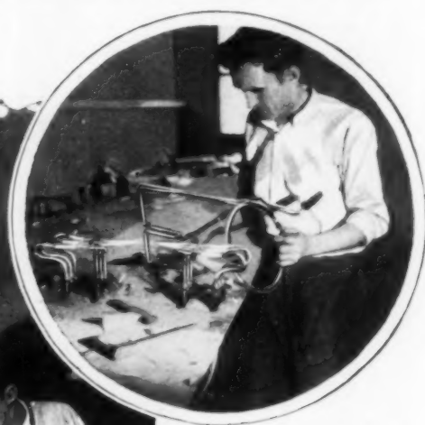
Left, Admitting Gas into the Tube; Above, Bending Tubing into Form of a Letter, and a Finished Word Assembly
