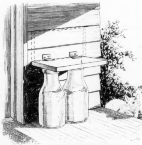
Hinged Board Prevents Cats and Dogs from Licking Tops of Milk Bottles
