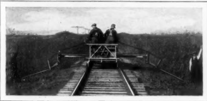
Keeping the Weeds in Check along the Railroad Right of Way; the Knives Reach Thirteen Feet on Either Side of the Track
