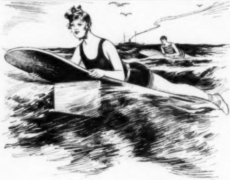
Buoyancy of a Surfboard Can Be Increased by Extra Board Hinged to the Bottom
