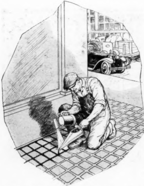
Conical Sheet-Metal Container for Tar, Which Facilitates Melting and Pouring It
