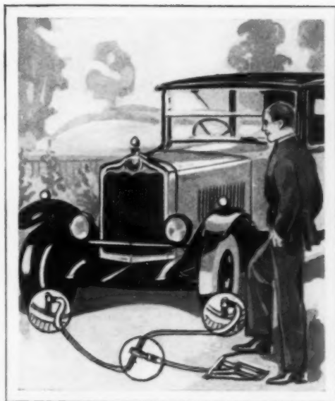
Pumping Both Tires at Once: Pressure Is Read on Gauge at Junction of Tubes
