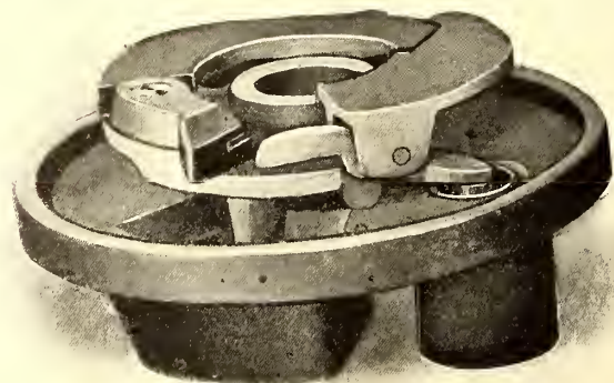
FIG. 4.—MOVABLE PORTION WITH ADJUSTABLE DASH-POT
