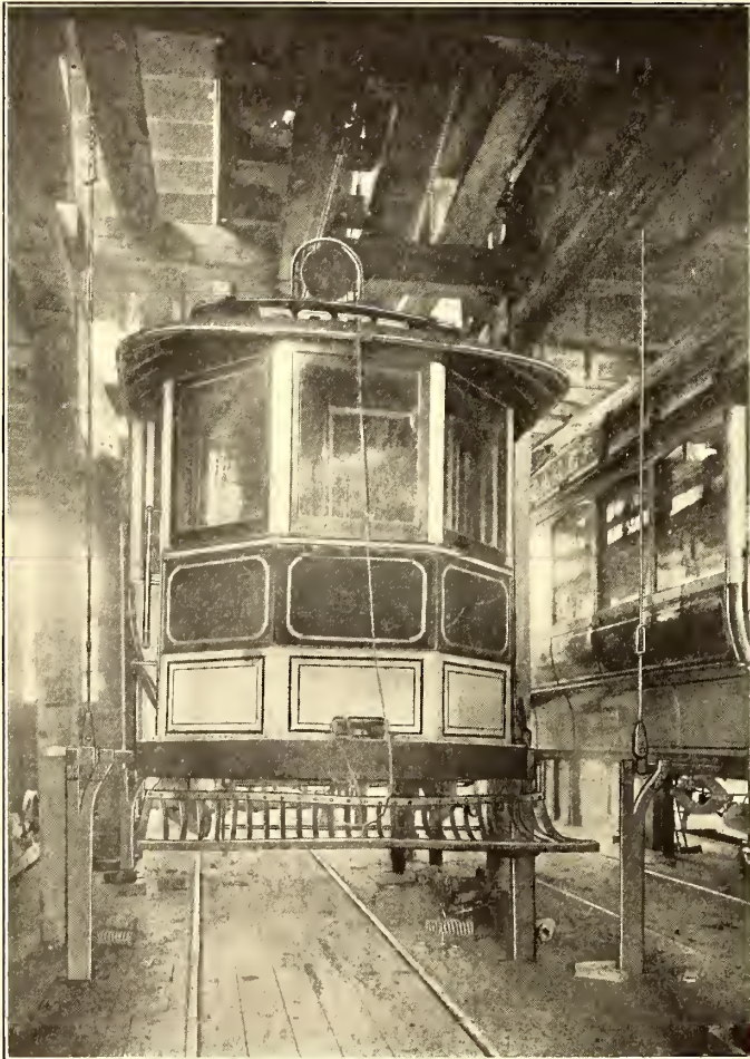
THE CAR HOIST IN THE TRUCK SHOP FOR LIFTING CAR BODIES OFF OF TRUCKS
