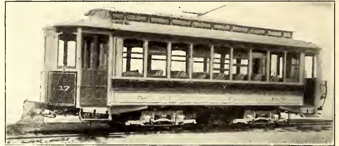
SEMI-CONVERTIBLE CAR USED IN THE VICINITY OF PHILADELPHIA
