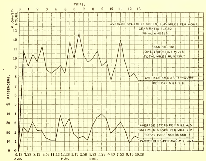
FIG. 5.—PASSENGERS AND KW-HOURS PER HALF TRIP, CAR NO. 101
