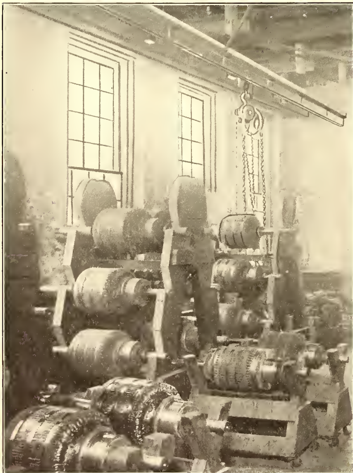
ARMATURE TRUCKS AND RACKS USED AT DETROIT
