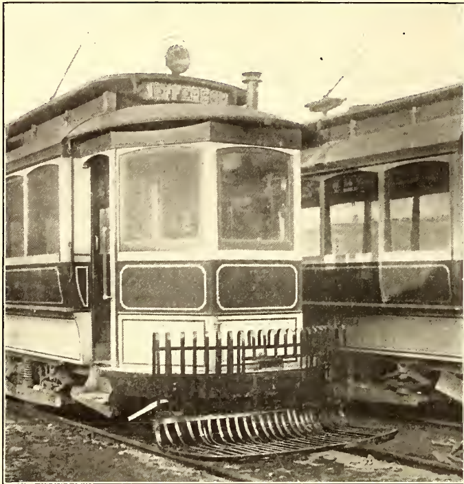
THE PRESENT FORM OF DROP-FENDER AS APPLIED TO ONE OF THE STANDARD CITY CARS OF THE DETROIT UNITED RAILWAY COMPANY
