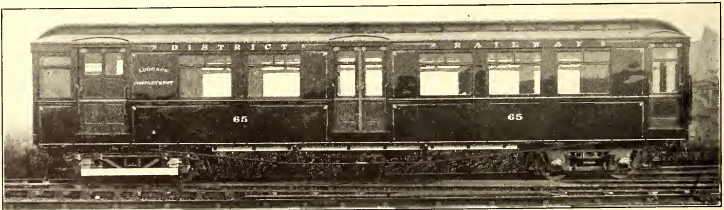
FIG. 68.—SIDE VIEW OF DISTRICT RAILWAY END MOTOR CAR WITH LUGGAGE COMPARTMENT
