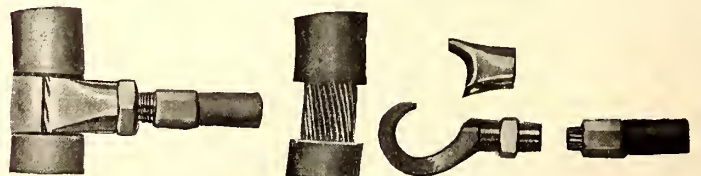
FIGS. 1 AND 2.—ASSEMBLY AND PARTS OF TAP JOINT
