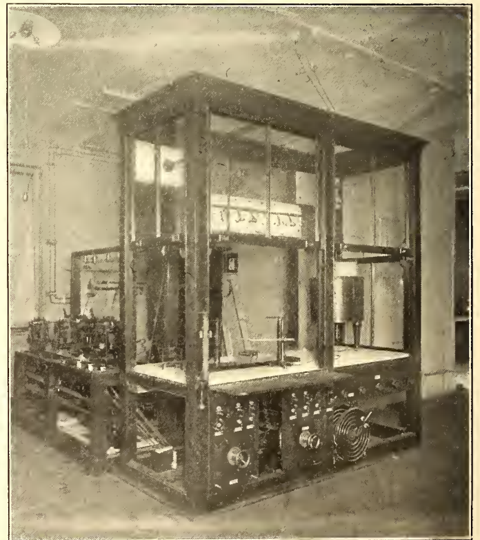
THE HIGH-VOLTAGE TESTING CABINET, WITH ITS EQUIPMENT OF GENERATORS, TRANSFORMERS, CONTROL AND MEASURING APPARATUS
