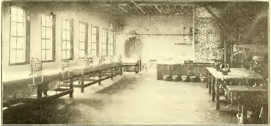
THE COIL-TAPING MACHINES AND AIR PRESSING MACHINES FOR FINISHING ARMATURE COILS
