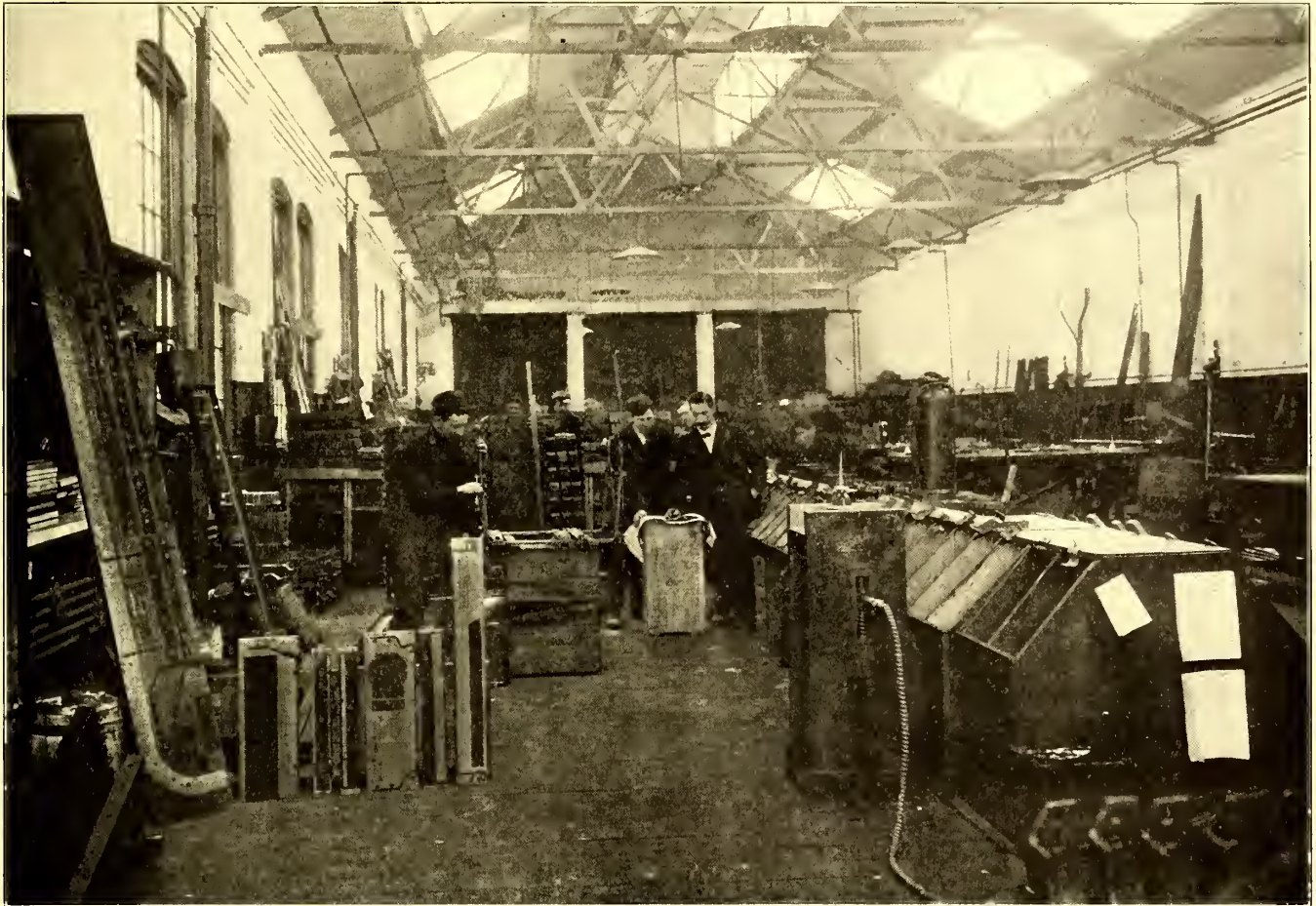
VIEW IN THE INSPECTION AND STOCK ROOM DEPARTMENT OF THE EQUIPPING SHOPS, SHOWING TEMPLATES FOR STANDARDIZATION OF ALL SPECIAL HANGERS, FITTINGS, ETC., USED
