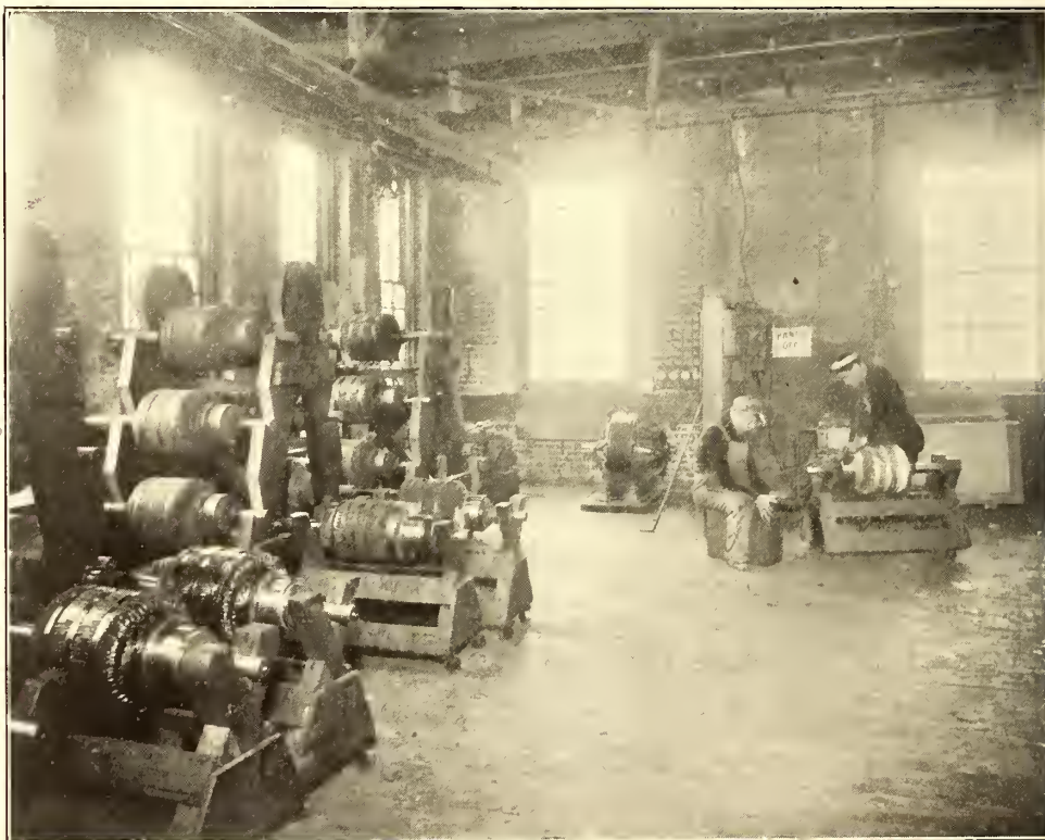
VIEW IN TESTING CORNER OF THE ELECTRICAL REPAIR DEPARTMENT, SHOWING ALSO SCHEME OF ARMATURE STORAGE IN USE
