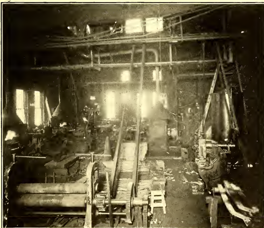
GENERAL VIEW IN THE BLACKSMITH-SHOP DEPARTMENT OF THE SHOPS, SHOWING ROLLS, PUNCHING MACHINERY AND POWER HAMMER
