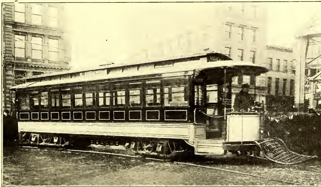
THE NEW TYPE OF CROSS-SEAT CONVERTIBLE SURFACE CAR, TO BE USED BY THE BROOKLYN RAPID TRANSIT COMPANY
