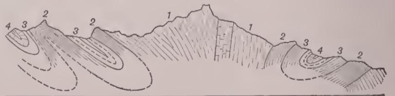
FIG. 3.—Section illustrating the fan-structure of the Alps (after Geikie). The numbers indicate different formations in the order of their original superposition, No. 1 being the lowest.
