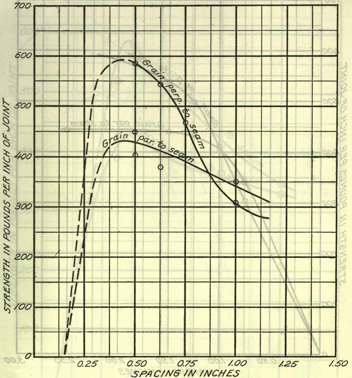
Fig. 35.—Multiple-riveted butt joints in plywood; relation between strength and spacing; test joint, 5 to 5 1/2 inches wide; margin, 1 inch; birch plywood, plies 1/20 by 1/20 by 1/20 inch; solid copper rivets, 0.15 inch diameter; sheet-metal cover plates; moisture, 5.6 per cent.
