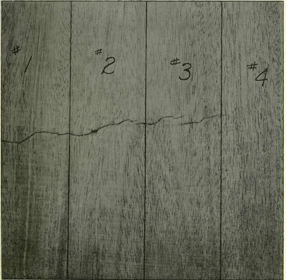
Fig. 16.—Compression failure occurring during growth. African mahogany
