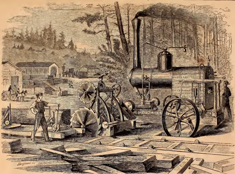
LANE & DODGE'S (OF CINCINNATI) PORTABLE STEAM CIRCULAR SAWMILLS.—SEE PAGE 345.
