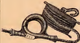
A "BREAK," THROUGH WHICH THE ROPES PASS, USED BY THE POMPER CORPS, TO REGULATE THE RAPIDITY OF THE DESCENT FROM ABOVE.
