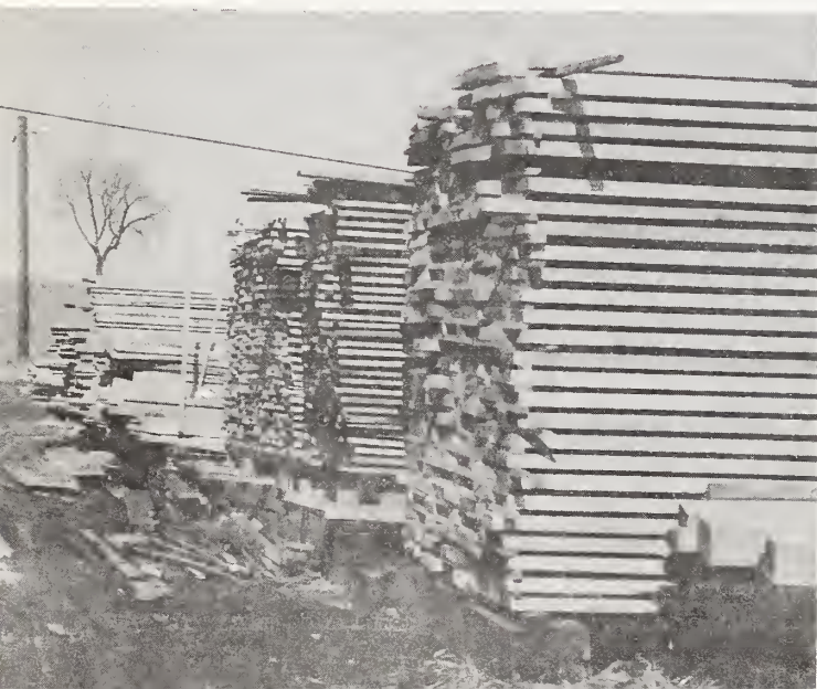
Figure 5.--This lumber has been graded, sorted, and stacked.
