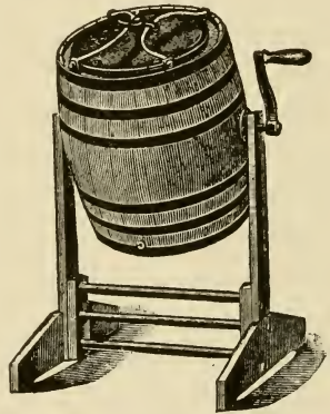
Fig. 34. The barrel churn. A modern tool for making home-made butter.
