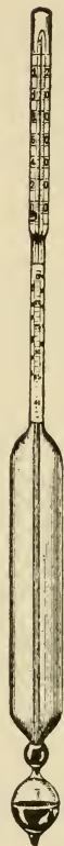
Fig. 28. Quevenne lactometer. The "dairy detective." It will show whether milk has been watered or skimmed, if used in connection with the fat test.
