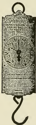
Fig. 41. Spring balance. The best scales for use in keeping milk and feed records of individual cows.
