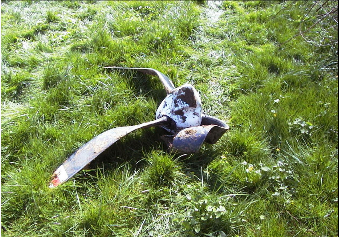
Figure C-3. Remains of the propeller (not in original position)
