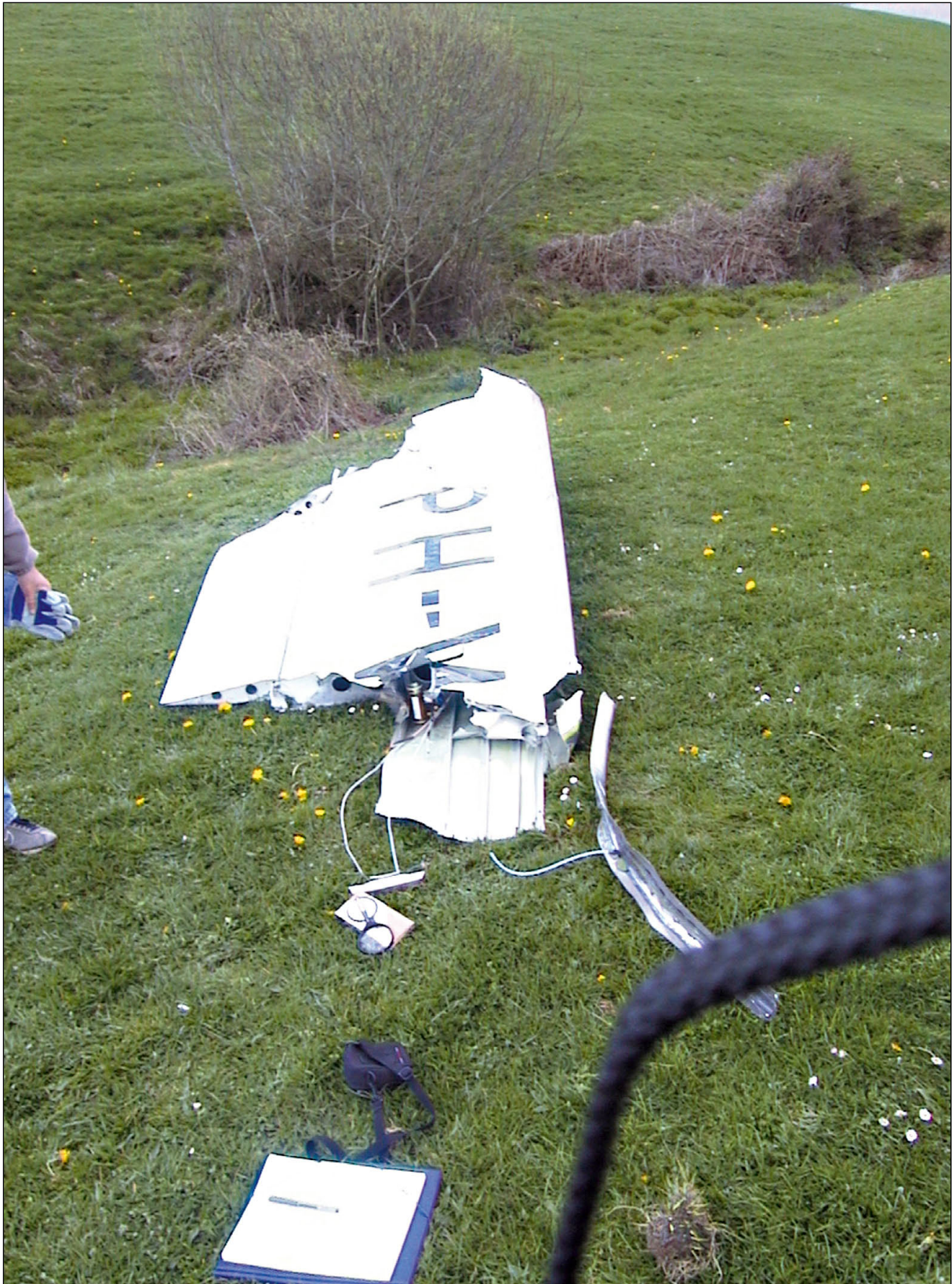
Figure C-6. Remains of the left inboard wing section
