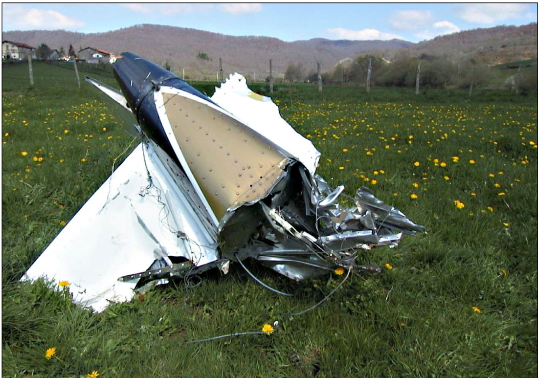
Figure C-4.2. Remains of the rear fuselage (seen from underneath)
