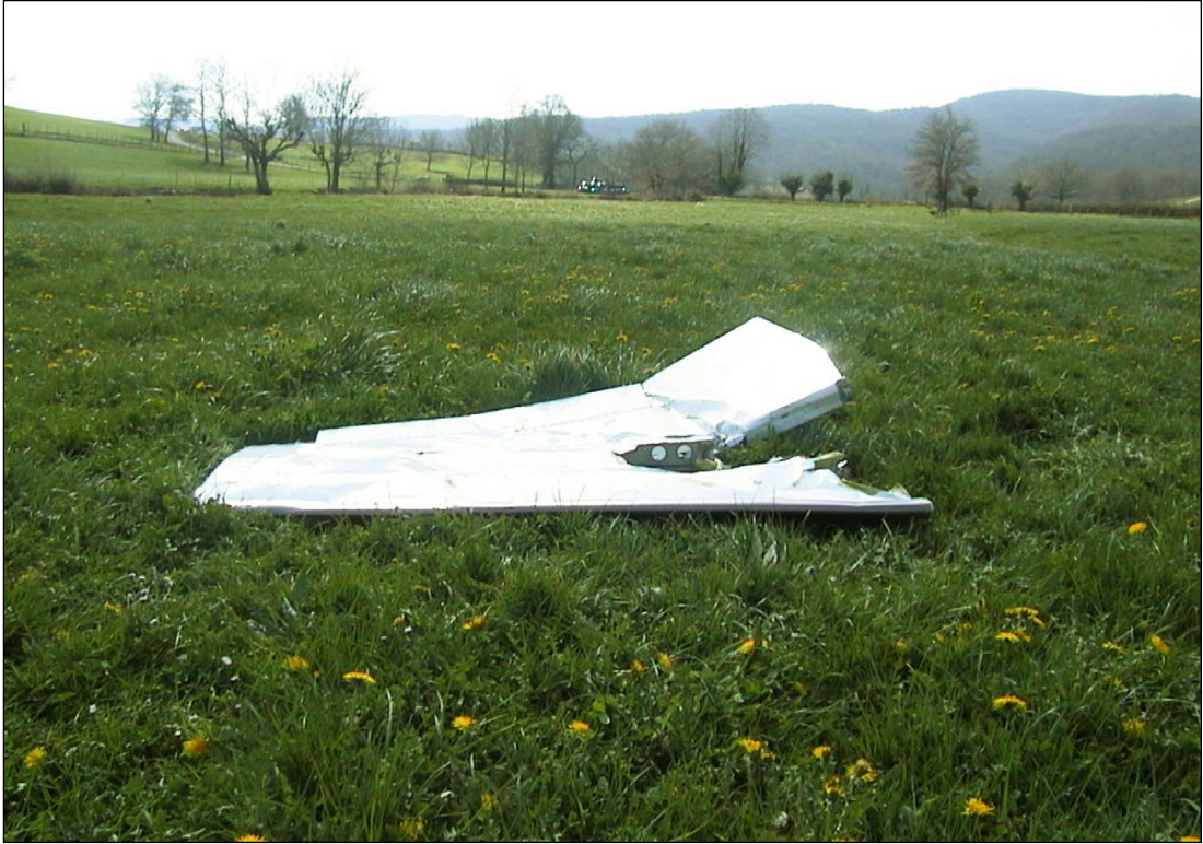
Figure C-5.1. Remains of the right stabilizer (inboard part)
