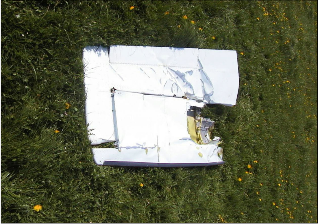
Figure C-5.2. Remains of the right stabilizer (outboard part)
