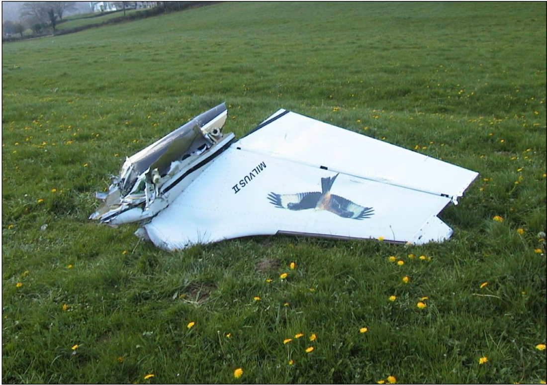
Figure C-4.1. Remains of the rear fuselage (view of the tail fin)
