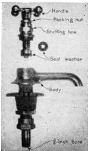
Figure 2.—Compression faucet for a washstand.
