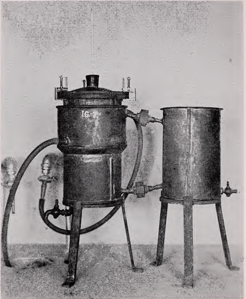
FIGURE 9.—Miniature 1-gallon percolator used for vanilla extraction. The finely cut beans are placed in a perforated container on the upper part of the percolator, and the solvent in the lower part. The temperature of the solvent is kept between 43° and 49° C. (109° - 120° F.) by means of the water jacket at the right.
