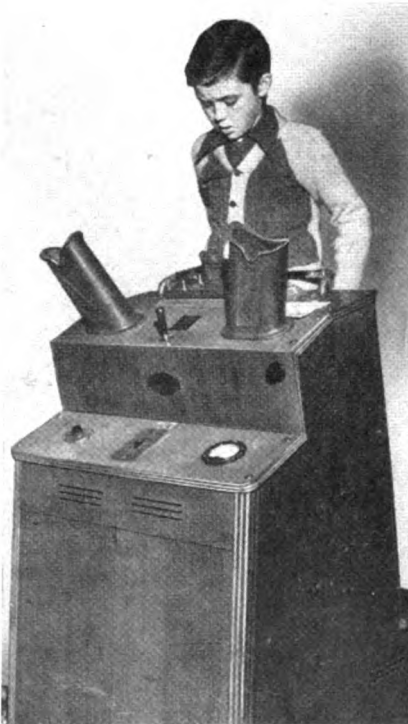
Millions of children and adults use the shoe-fitting fluoroscope machines, now the subject of many investigations to determine the health hazards from stray radiation and electrical shock.
