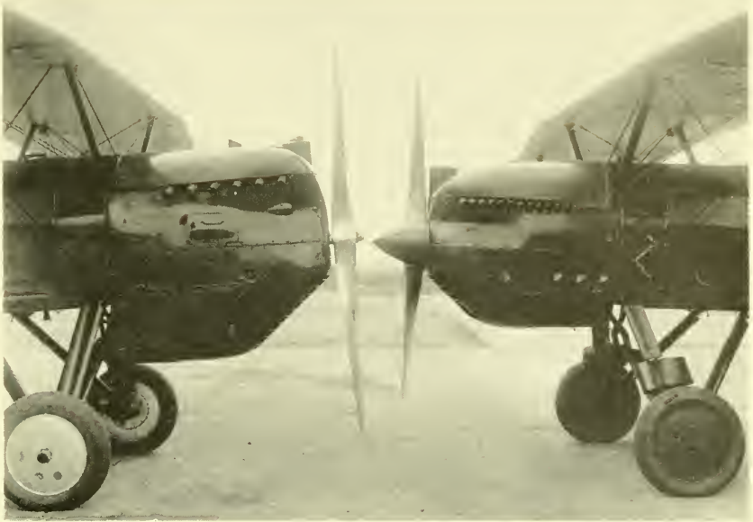
1. Comparison of radiator installations for water (left) and Ethylene Glycol cooling, on Curtiss Falcon airplanes, 1930. (Courtesy Curtiss-Wright Corp.)
