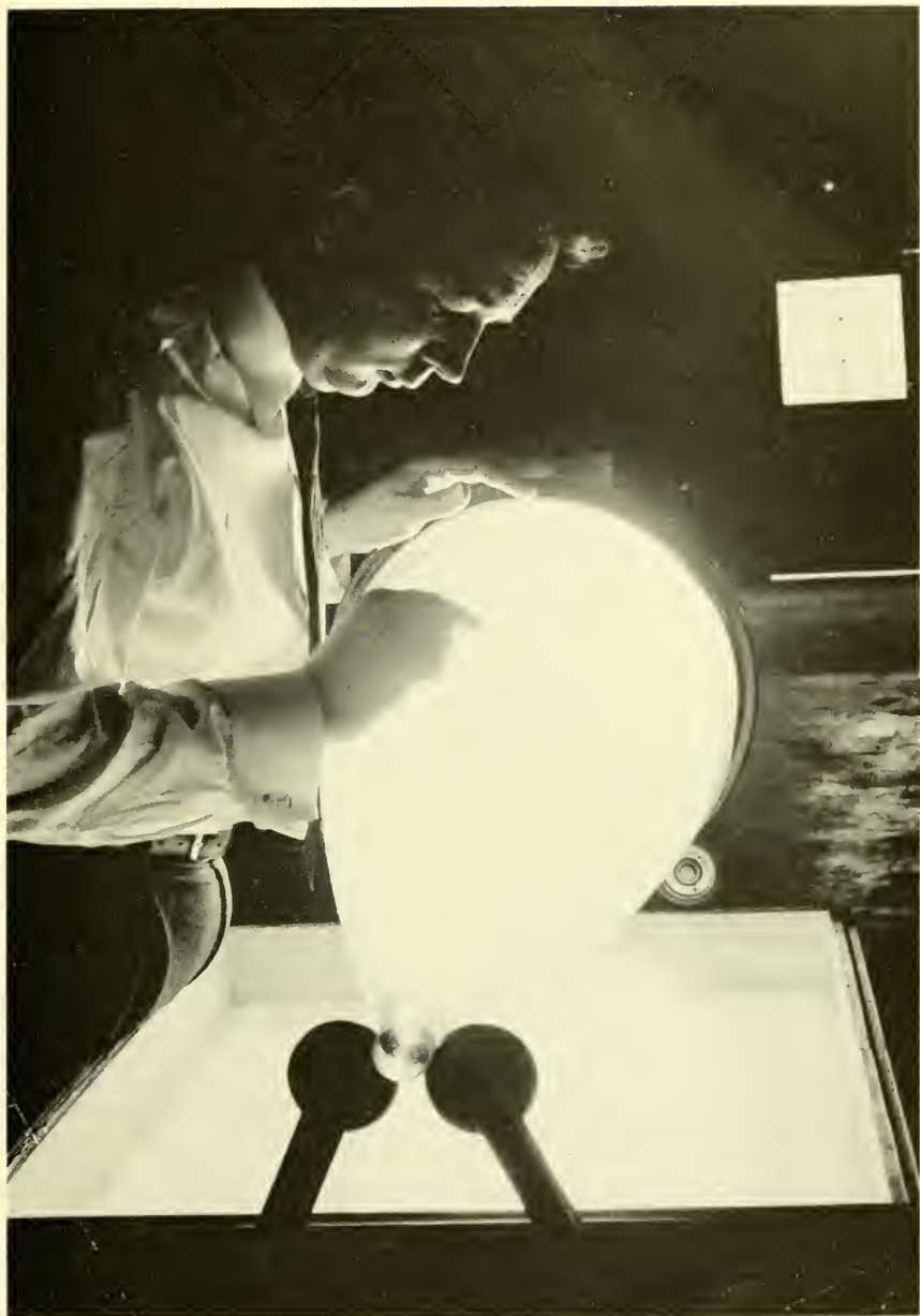
One of the new glasses that can be changed to crystallized glass-ceramic. Here it is shaped into a missile nose cone. In its transparent glassy state, undergoing inspection at right, it is ready for heat treatment to form millions of tiny nuclei and cause crystals to grow on these centers. The matured glass-ceramic has great resistance to erosion and thermal stress.
