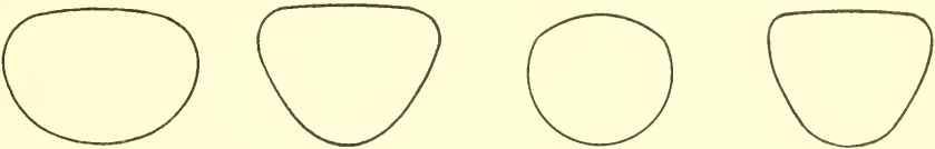
FIGURE 3.—Typical shapes of cross sections of limbs of traditional longbows.
