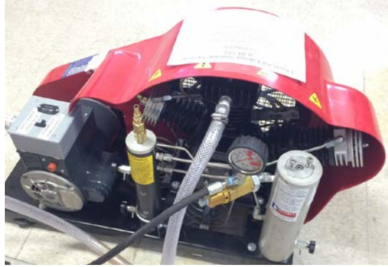
Figure 4. AireTex 45 Oil-Free Air Compressor as Part of the Nitro-Turbodyne LAES System. Source: Nitro-Turbodyne (2016b).
