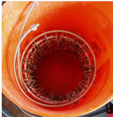
Figure 5. Ice-Water Heat Exchanger
