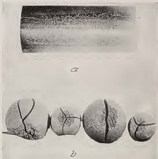
FIG. 10.— Mechanical nonuniformity of wrought metals revealed by deep etching
