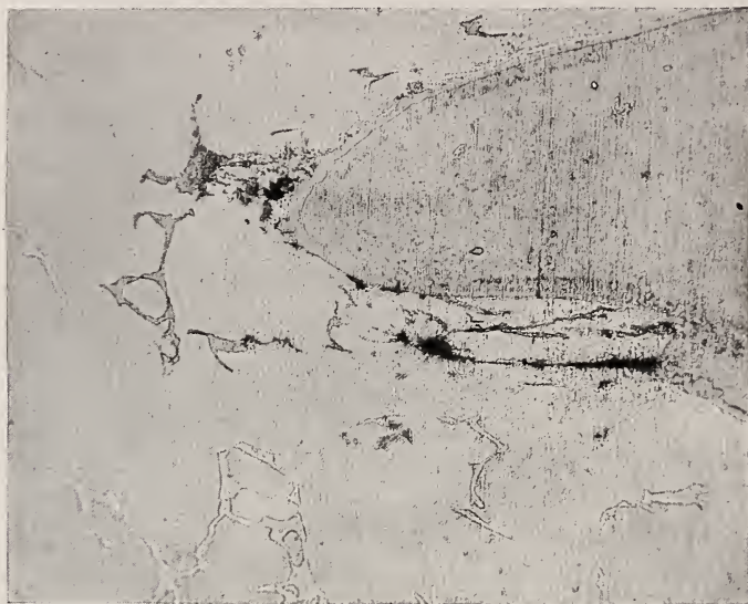
FIG. 63.—Microstructure of corroded Muntz metal, illustrating the effect of stress in localizing the corrosive action of this alloy. \times 250
