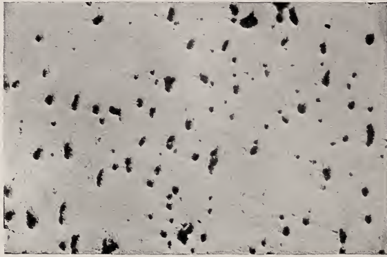
FIG. 69.—Microstructure of leaded brass. \times 100
