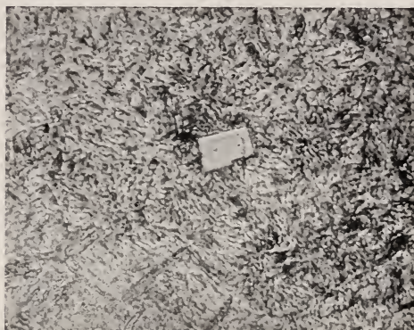
FIG. 17.— Characteristic appearance of an inclusion caused by the addition of titanium to steel. X 1000
