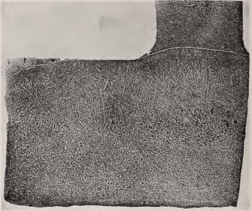
FIG. 3.—Macrostructure of a defective steel casting revealed by deeply etching with hot concentrated hydrochloric acid. \times 1/2
