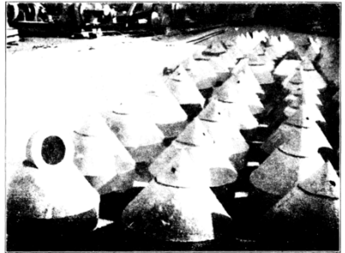
IRON SHOES FOR CONCRETE PILES.
