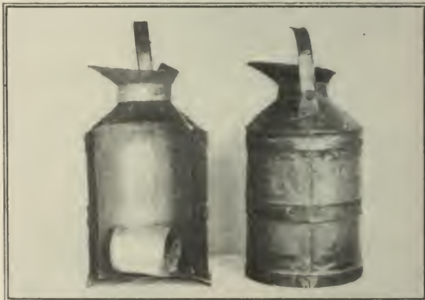
A "FIVE-GALLON" CAN CONTAINING SMALL CAN WHICH IS DRAWN UP BY A STRING TO THE OPENING AND MADE TO DO DUTY
