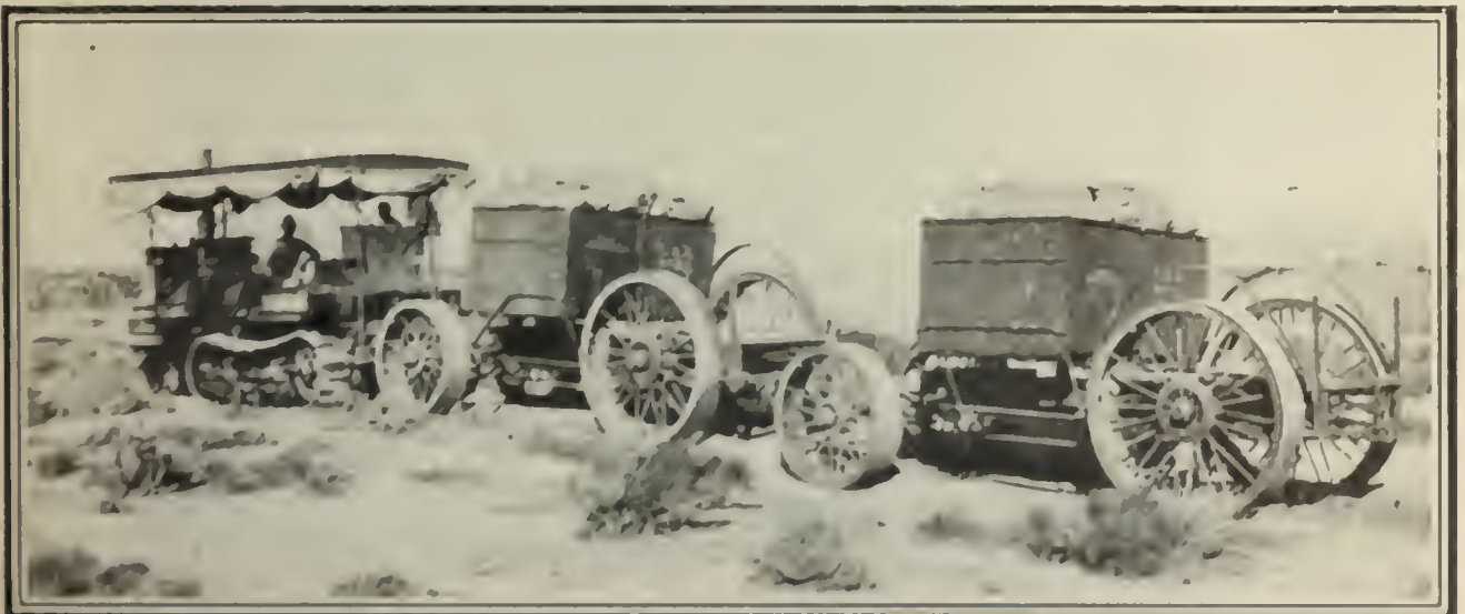
CATERPILLAR TRACTION ENGINE, HAULING ROCK FOR CONCRETE, ACROSS THE DESERT
