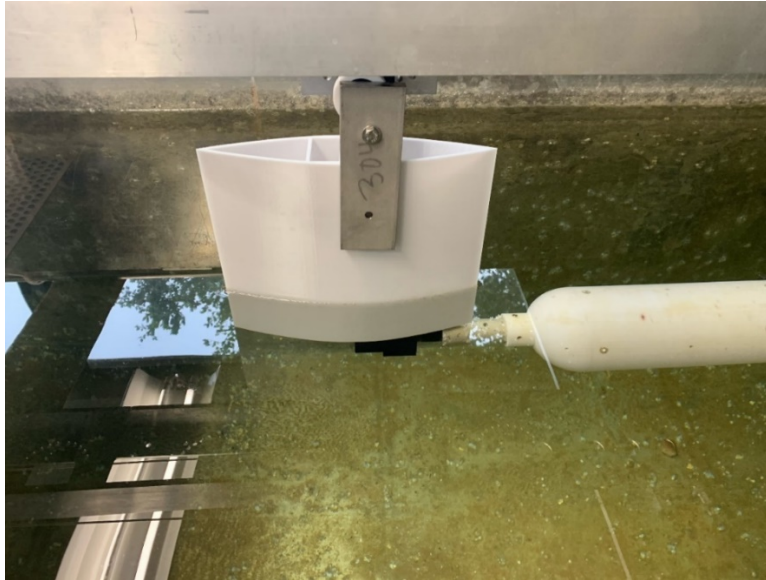
Figure 11. Fairing installed around sting
