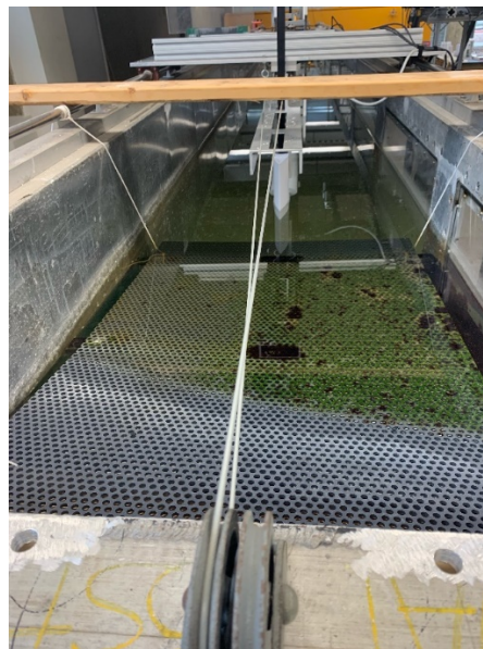
Figure 8. Beach made out of perforated acrylic sheets
