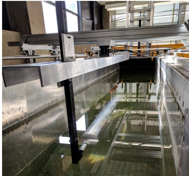
Figure 10. Sting style test fixture with model attached. Source: [5].
