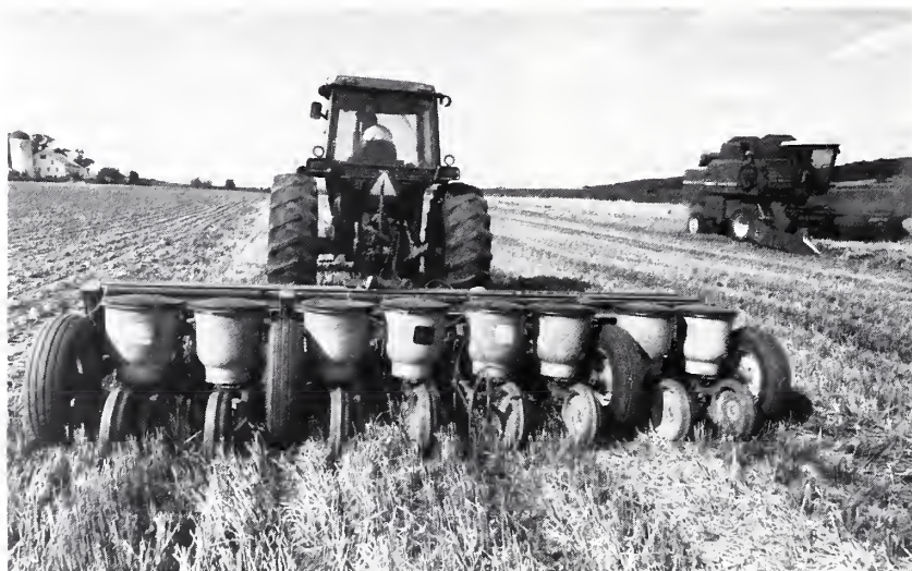
No-till planting—a new crop in the residue of the harvested crop in Carroll County, Md.
