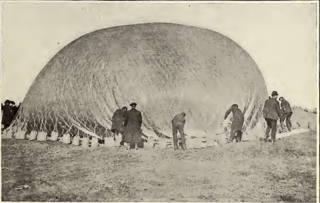
AS THE BAG FILLS, MEN WALK AROUND THE BALLOON SHIFTING THE BAGS TO LOWER LOOPS OF THE CORDAGE.
