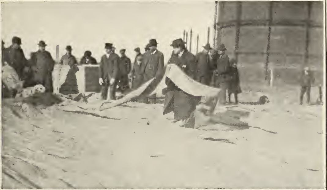
WALKING ON THE BALLOON TO GET TO THE VALVE-HOLE. THE AÉRONAUT CAREFULLY LAYS A STRIP BEFORE HIM TO PROTECT THE FABRIC FROM BEING TORN OR INJURED BY HIS SHOES.
