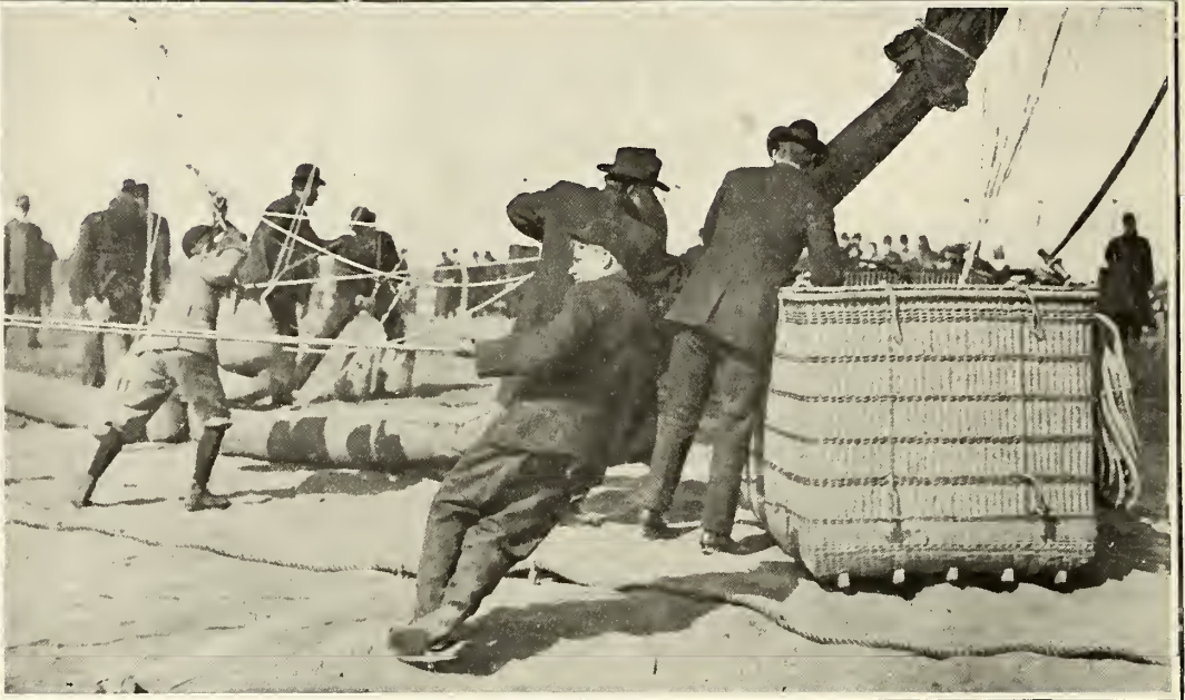
STILL PULLING IN THE CORDAGE TO NARROW IT DOWN TO THE BASKET. THIS PICTURE GIVES A GOOD VIEW OF THE FILLING-PIPE OF THE BALLOON THROUGH WHICH THE GAS IS POURING INTO IT.
