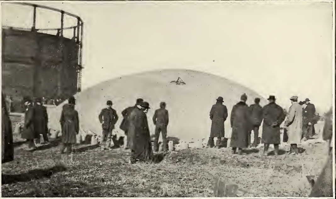
THE GAS IS FILLING THE BALLOON SLOWLY. THE VALVE IS SHOWN NEAR THE TOP.
