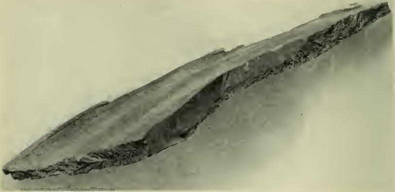
Section of turbine disc which exploded because of a fatigue crack.
