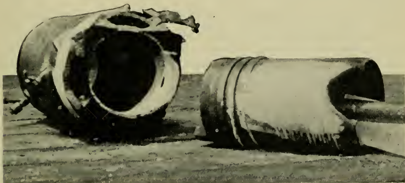
Figure 8—Piston and part of cylinder which broke off due to over-heating. The machine was a small two-cylinder engine.
