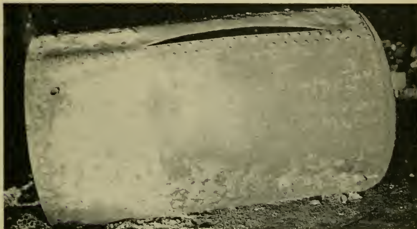
Lap seam crack inconveniences utility.
