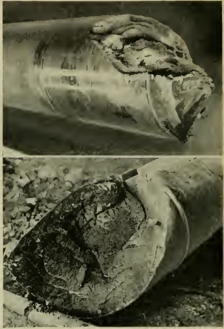
Result of progressive crack in 15" shaft.
