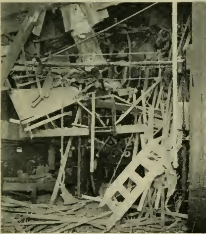
Cotton compress after explosion of its steam cylinder.
