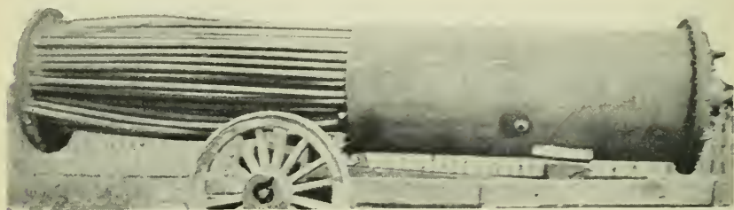
Fusion welded ammonia condenser which failed; welding procedure and testing have advanced greatly since this vessel was built.
