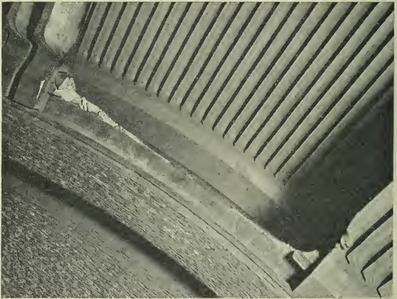
Figure 1—The broken disc. The dovetail arrangement of fastening the blades is clearly visible at the left.
