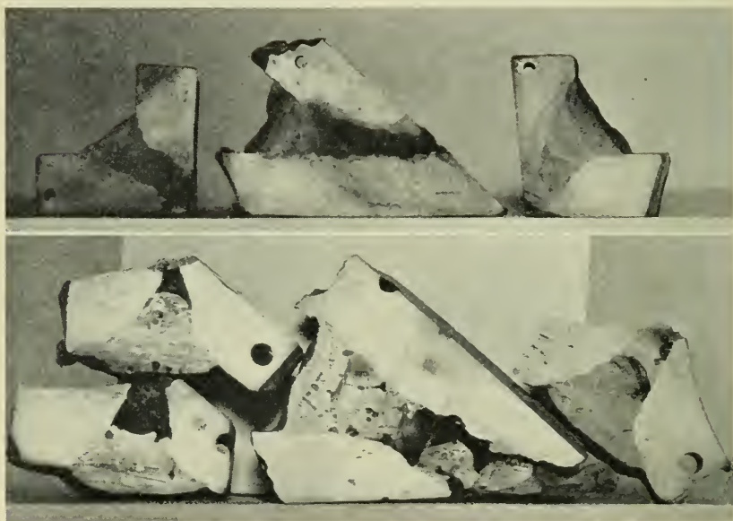
Good and bad fusion in pipe joints.
