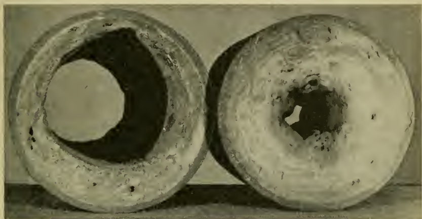
An extreme example of scale in boiler tubes.
