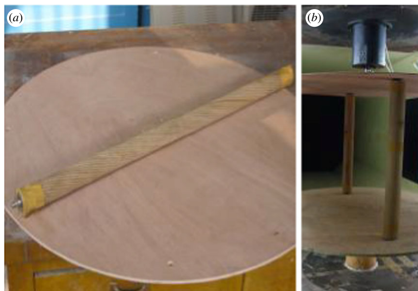
Figure 4. Wind tunnel test model. (a) A sub-conductor model. (b) Twin bundle conductor model.
