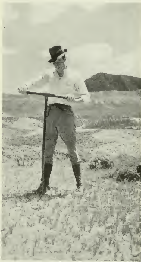
NO ROCK HERE The earth auger tests the soil to the depth which the plow will penetrate
