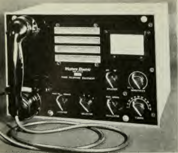
FIG. 4. This ship's radio telephone set, made by the Western Electric Company, provides conversation channels on four frequencies
