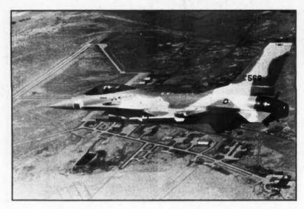
The Air Force's F-16 program is a minimum risk and minimum overall cost program; it achieves important commonality with the F-15 through use of a common turbo-fan Pratt and Whitney engine having excellent fuel consumption characterics.
