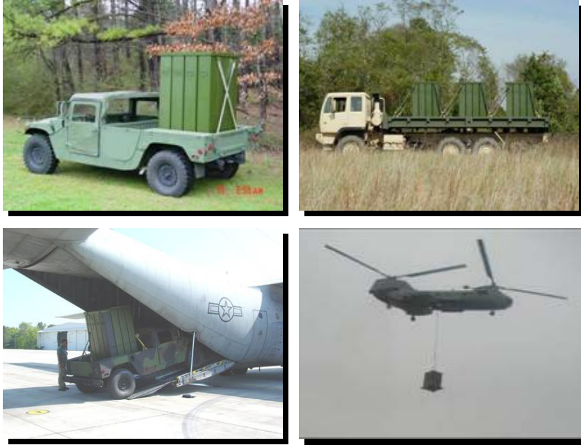
Figure 1: NLOS-LS Platform Independence 6 . The flexibility of the launcher allows interoperability among various manned/unmanned platforms. The system can be launch on a M998 High Mobility Multipurpose Wheeled Vehicle (HMMWV) and deployable by a C130 aircraft.
