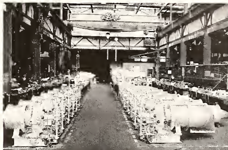
A Shipment of Turbo Propeller Forced Draft Blowers made for Destroyer Service by B. F. Sturtevant Co.
