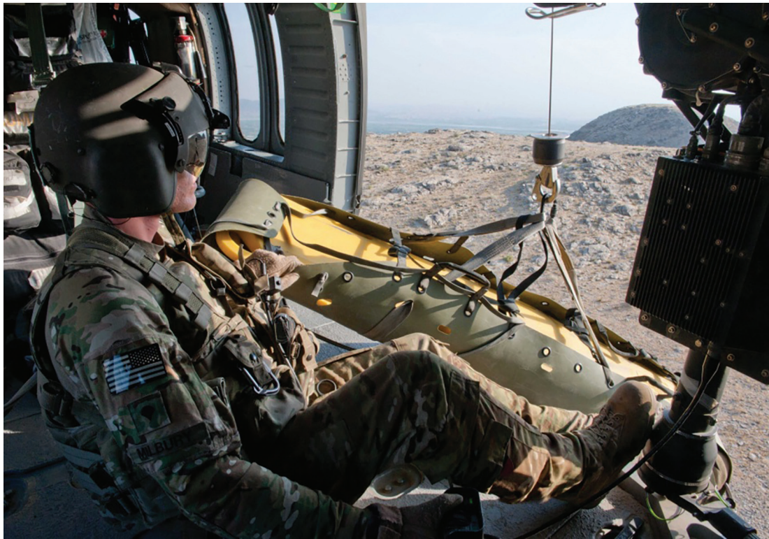
FIGURE 13.5. MEDEVAC crew chief with hoist near Forward Operating Base Fenty, Nangarhar province, Afghanistan, September 16, 2013. Using a hoist allows MEDEVAC crews to raise injured warfighters from remote or treacherous areas where landing the aircraft is impossible. US Army National Guard photo by Sergeant Margaret Taylor, 129th Mobile Public Affairs Detachment/RELEASED. Reproduced from: https://www.dvidshub.net/image/1023428/dustoff-medevac-crew-polishes-rescue-skills .
