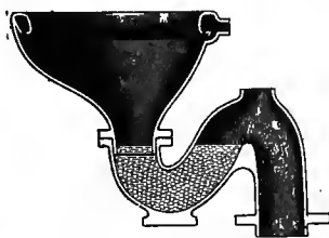
Short Hopper Section Showing Seal.
