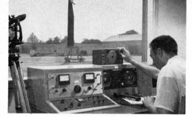
Electronics Research Engineer Irving Alne records radiation antenna patterns on Lockheed's Radar Range. Twenty-two foot plastic tower in background minimizes ground reflections, approximates free space. Pattern integrator, high gain amplifier, square root amplifier and logarithmic amplifier shown in picture are of Lockheed design.
