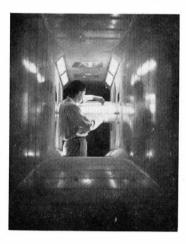
C. H. Fish, design engineer assigned to Lockheed's Icing Research Tunnel, measures impingement limits of ice on C-130 wing section. The tunnel has a temperature range of  $-40^{\circ}\mathrm{F}$ . to  $+150^{\circ}\mathrm{F}$ . and maximum speed of more than 270 mph. It is the only icing research tunnel in private industry.
