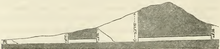
A vertical section of the upper portion of the culvert at Seleucia Pieria, as surveyed by Capt. W. Allen, R.N.
