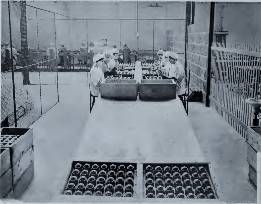
Filling the Base Charge and Packing No. 80 Fuse
