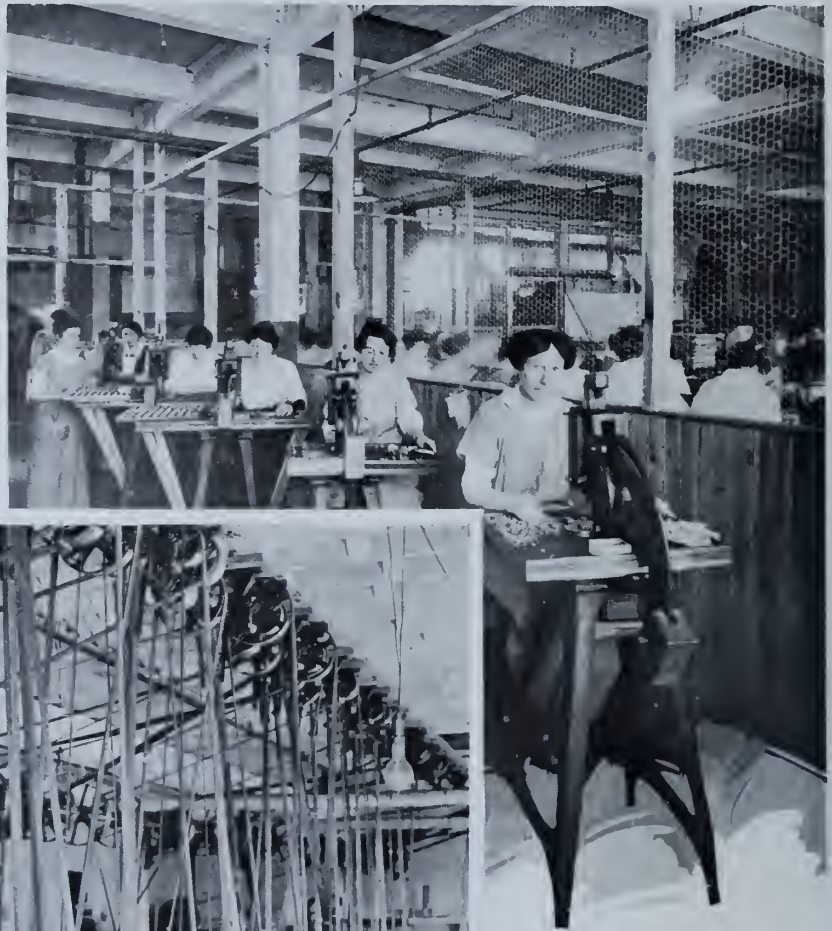
Foot Presses. Pressing Needles in Needle Plug.
