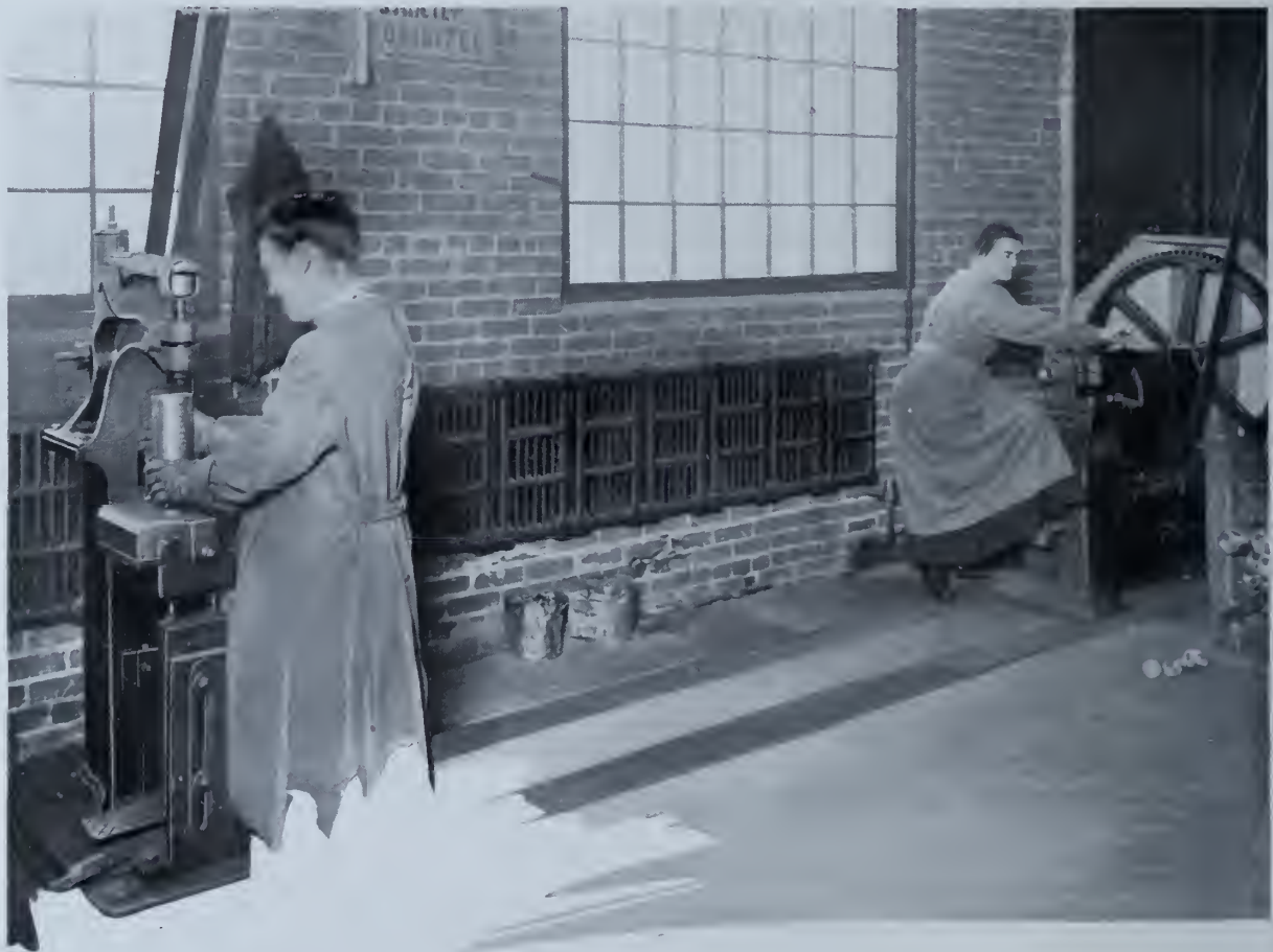
Screwing in the Base Plate and Rivetting ditto, 18-pounder High Explosive Shells
