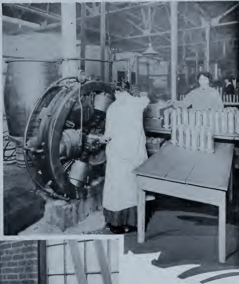
Pressing on the Copper Driving Band with Hydraulic Press
