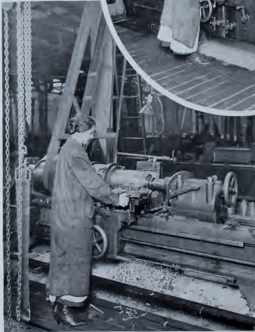
Undercutting and Waving of 8 inch Shells
