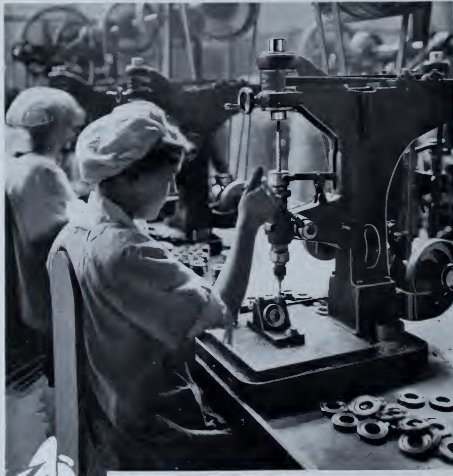
Detail of Drilling Operation, Clearly Showing the Jig and its Usefulness
