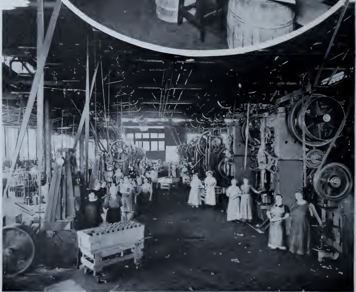
General View of Shop and Bank of Power Presses on Cartridge Cases for 18 Pounders.
