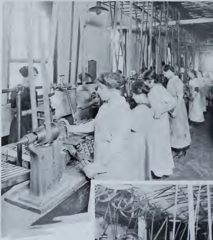
Milling the Undercut of Flash Hole in Stem No. 80 Fuse
