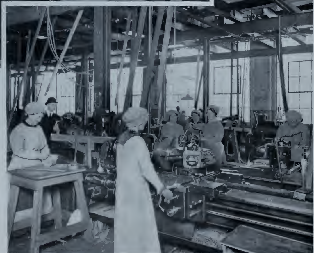
Rough turning the Adaptor Second operation
