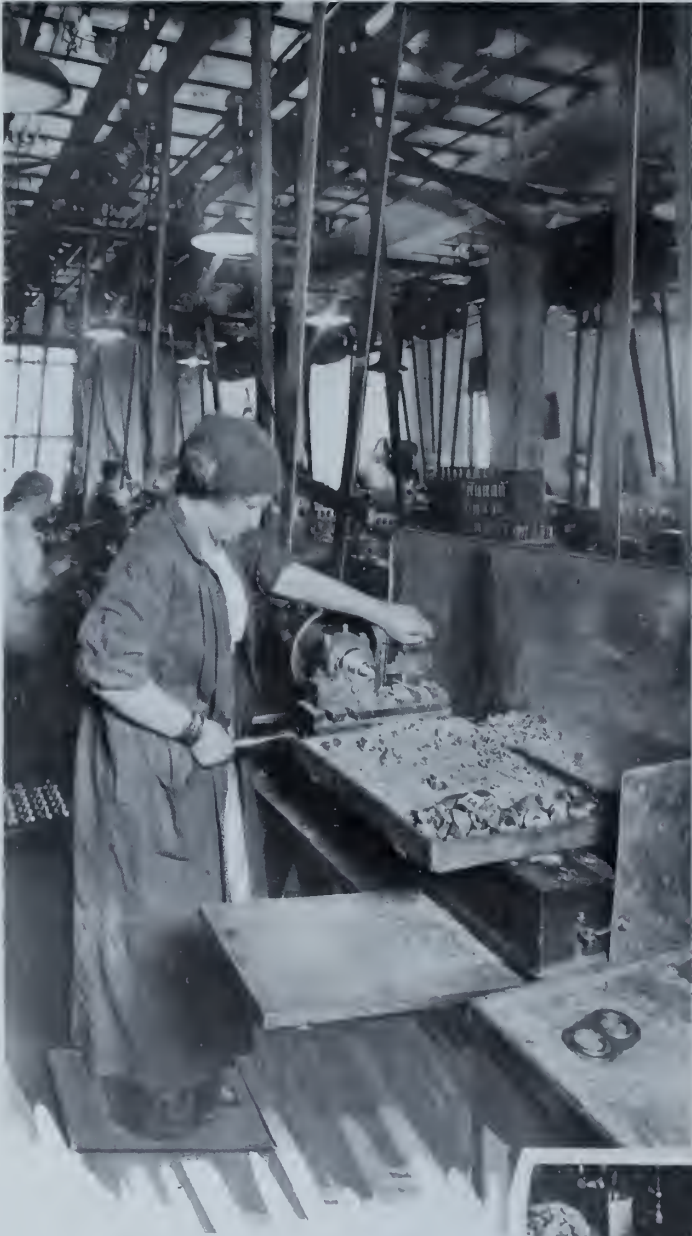
Rough and Finish Turning of Cap No. 80 Fuse
