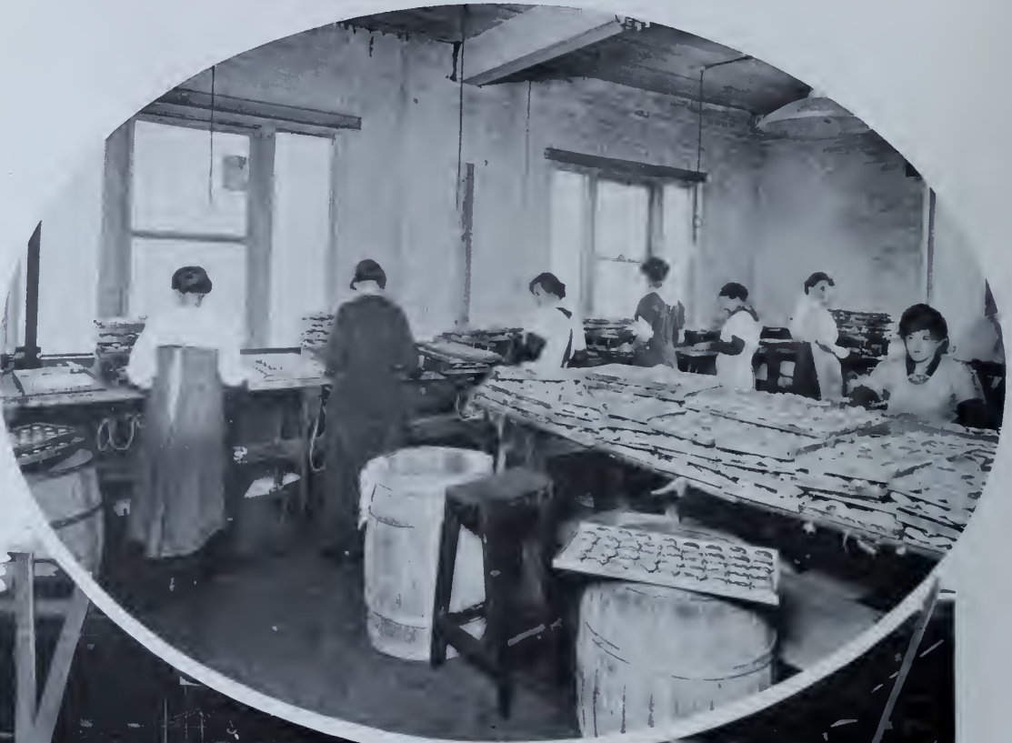
Soldering Powder Cans for 18 Pounder Shrapnel Shells.
