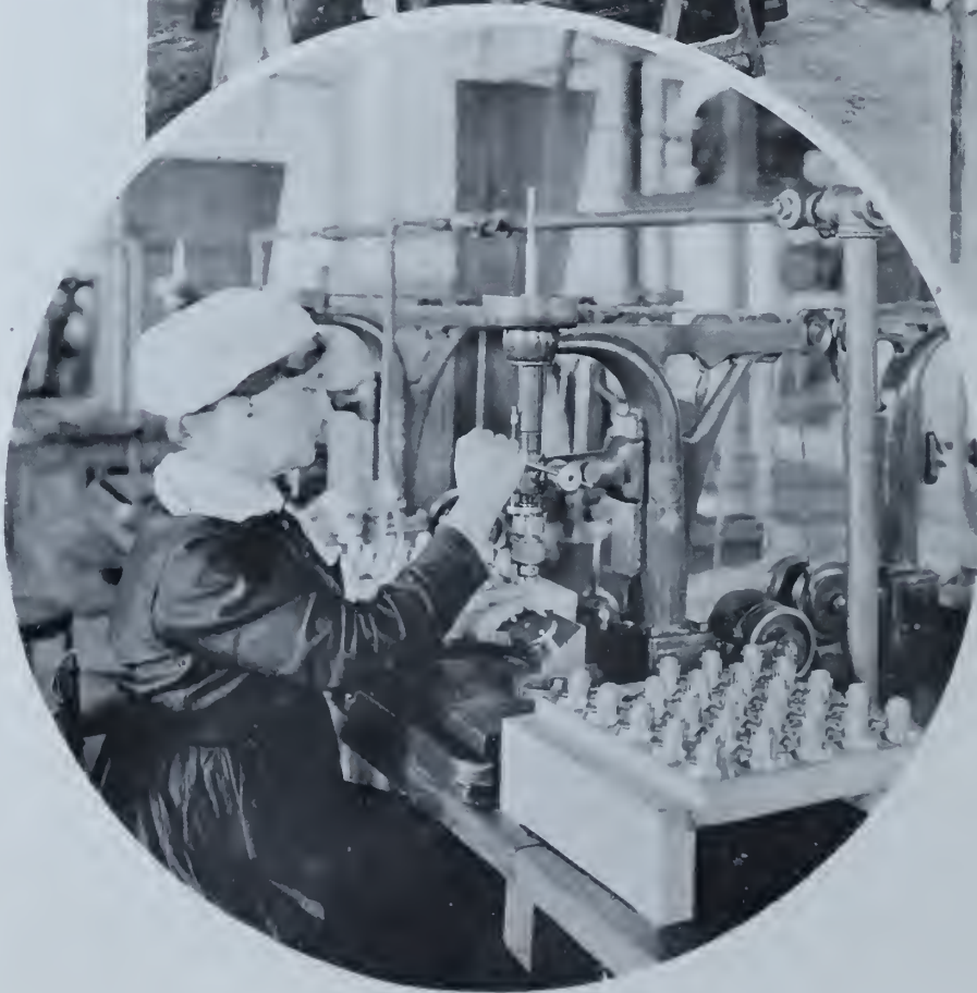
Drilling the Flash Hole No. 80 Fuse
