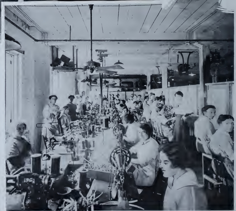
Tacking and Closing Assembling Strips for Cartridge Case Clips
