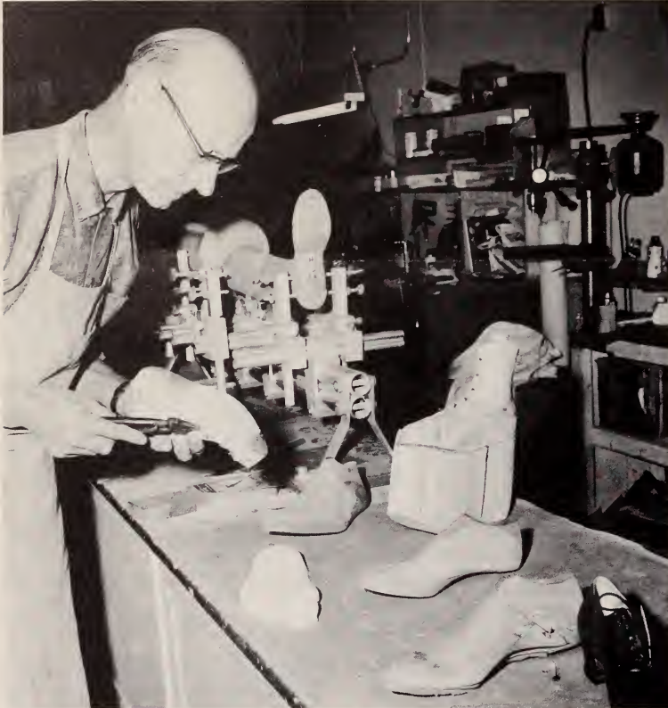
Skilled orthopaedic specialists carefully construct artificial limbs and braces at Canada Limb and Brace Limited in Edmonton. Above, different types of shoes in various stages of completion, with complex limb alignment machine for accurate form measurements in background.
