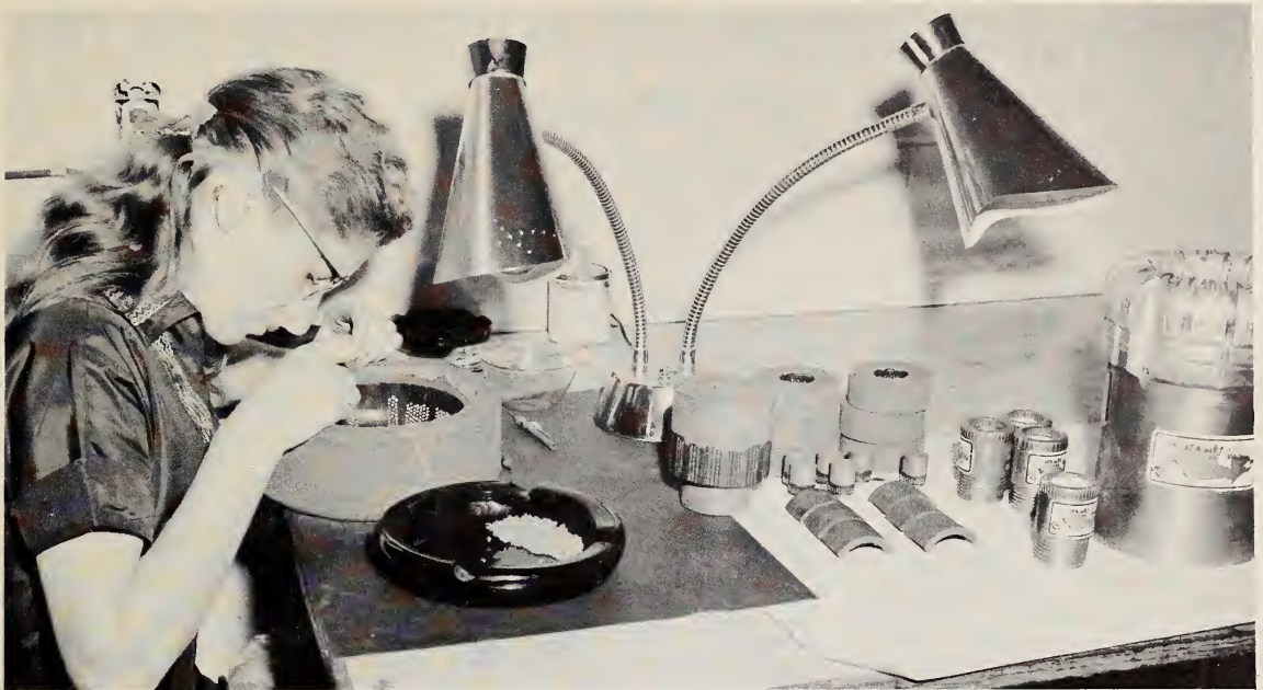
Industrial diamonds (in ash tray) are placed in mould by hand at Canada Bit Limited in Edmonton. Various size bits and several moulds are on table. Bits are made by powdered metallurgical process in a furnace heated to 2,000 degrees Fahrenheit.
