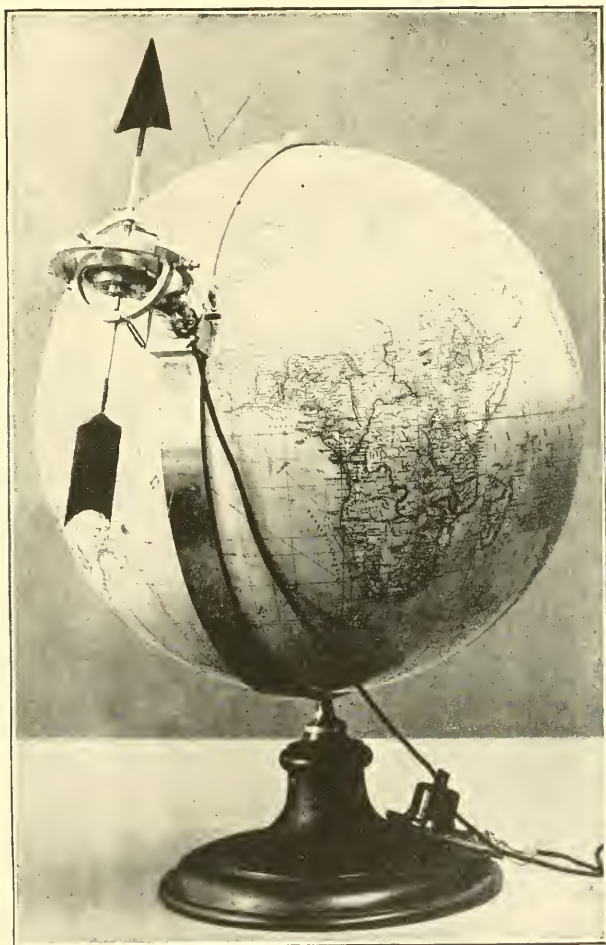
DEMONSTRATION MODEL OF GYROSTATIC COMPASS.
