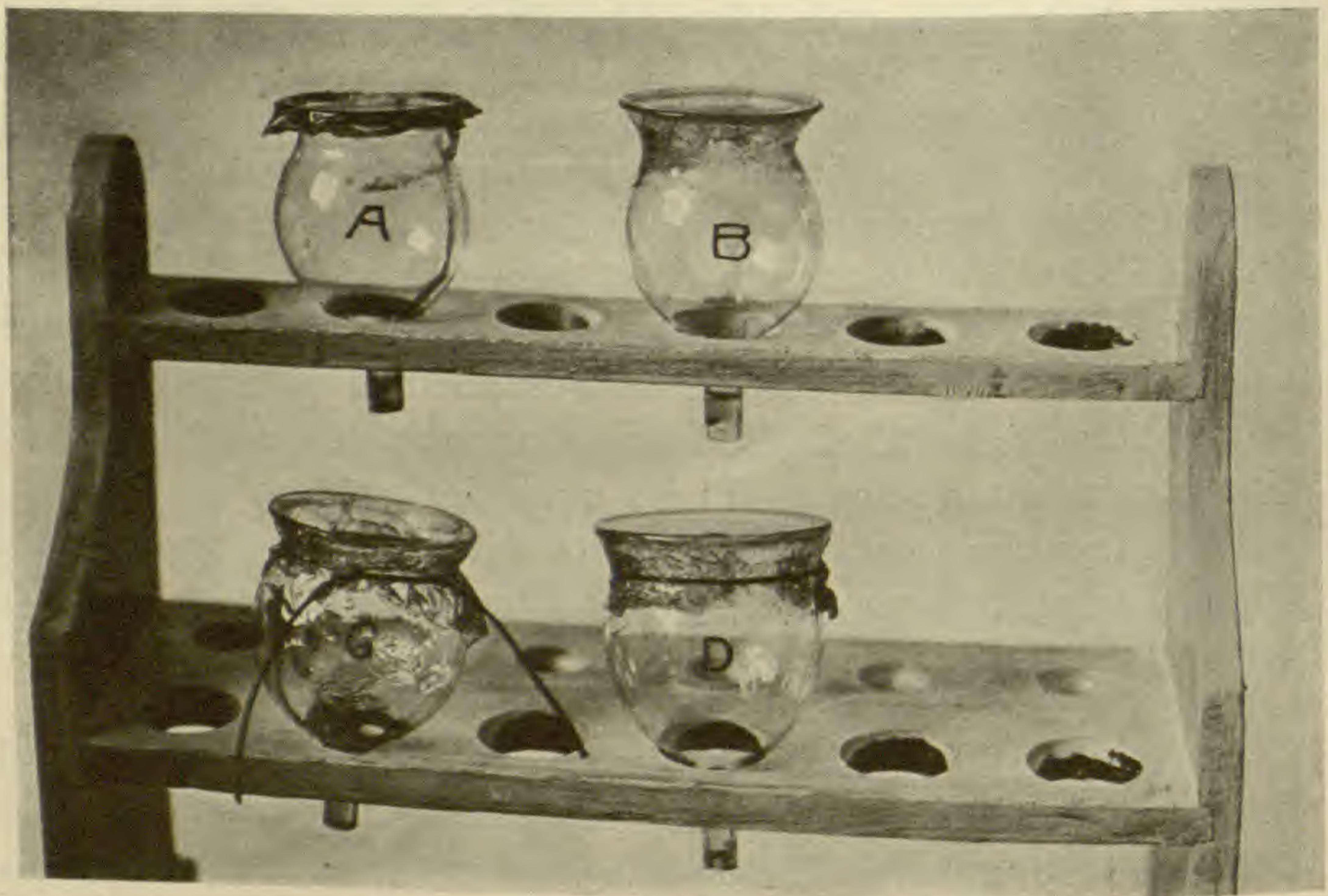
FIG. 2.—Different stages in the formation of celloidin membranes: A , membrane after being placed over the bulb of a thistle tube; B , showing how the film adheres to the flange; C , after tying the membrane on the thistle tube; D , a double membrane.
