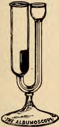
Fig. 300.—The Horismascope or Albumoscope. A new instrument for determining the presence and amount of albumin in the urine. No liability of the acid mixing with the urine. The slightest visible trace of albumin can be instantly detected against the dark background. Color reactions due to urinary and biliary pigments are clearly shown against the white background.
